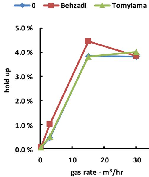
Figure 8: Gas hold up in narrow vessel for different lift expressions as function of gas rate.
