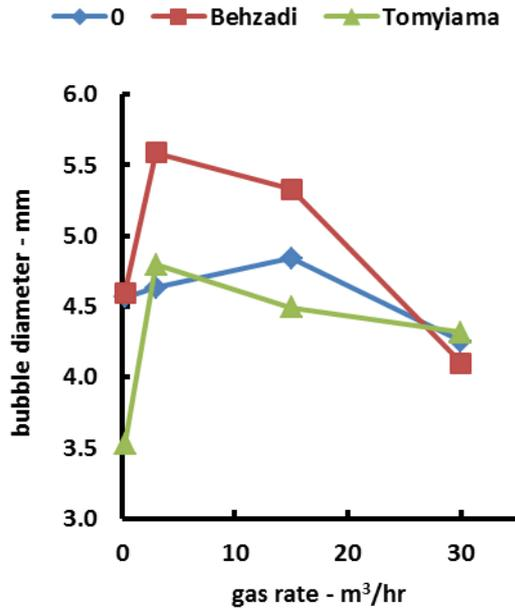
Figure 12: Bubble diameter in narrow vessel for different lift expressions as function of gas rate.
