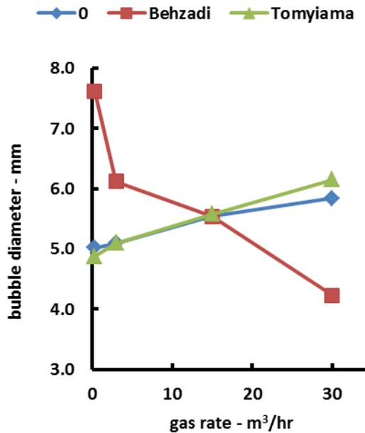
Figure 13: Bubble diameter in wide vessel for different lift expressions as function of gas rate.
