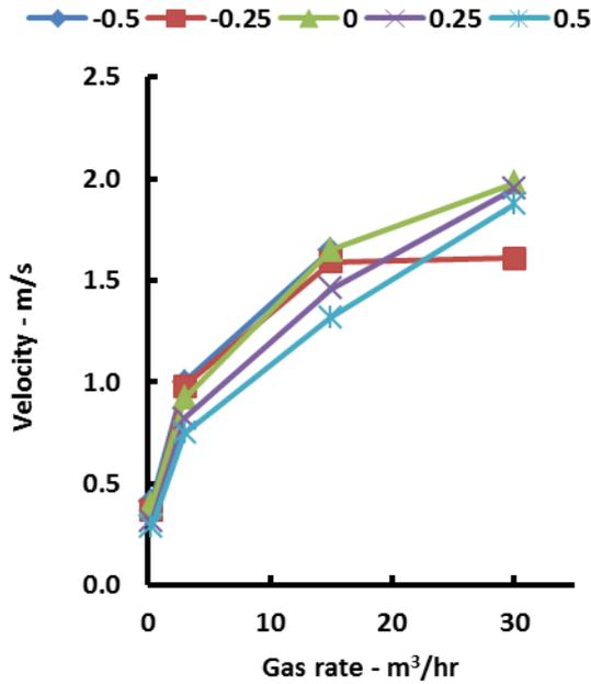
Figure 6: Centre velocity for different lift coefficients as function of gas rate for the narrow vessel.
