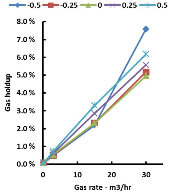
**Figure 4:** Gas holdup for different lift coefficients as function of gas rate for the narrow vessel.
