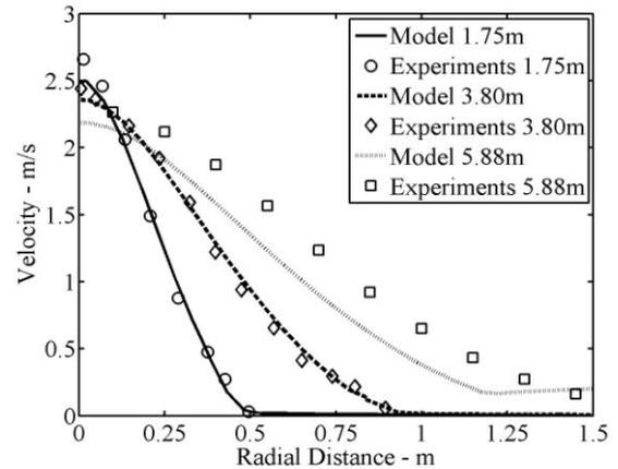
**Figure 1:** Modelling results of velocity profiles of the liquid phase at different heights above gas release point compared with experiments at a gas rate of 170 NI/s.
