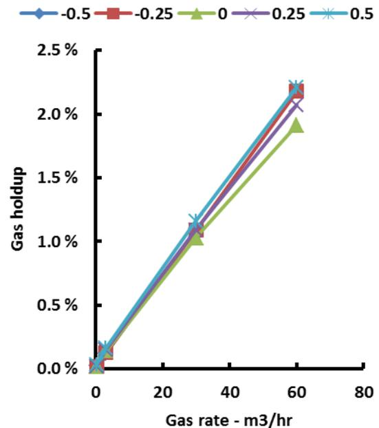
**Figure 5:** Gas holdup for different lift coefficients as function of gas rate for the wide vessel.
