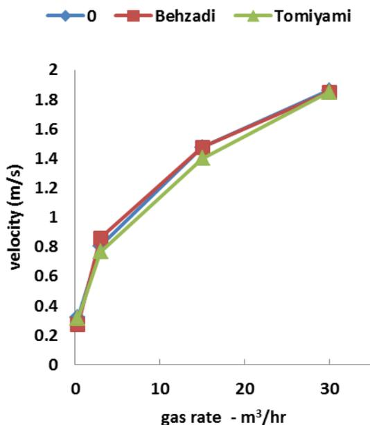
Figure 11: Centre velocity in wide vessel for different lift expressions as function of gas rate.
