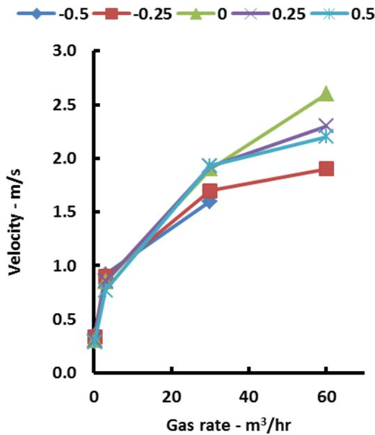
Figure 7: Centre velocity for different lift coefficients as function of gas rate for the narrow vessel.
