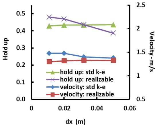
**Figure 3:** Grid dependence and effect of turbulence model
