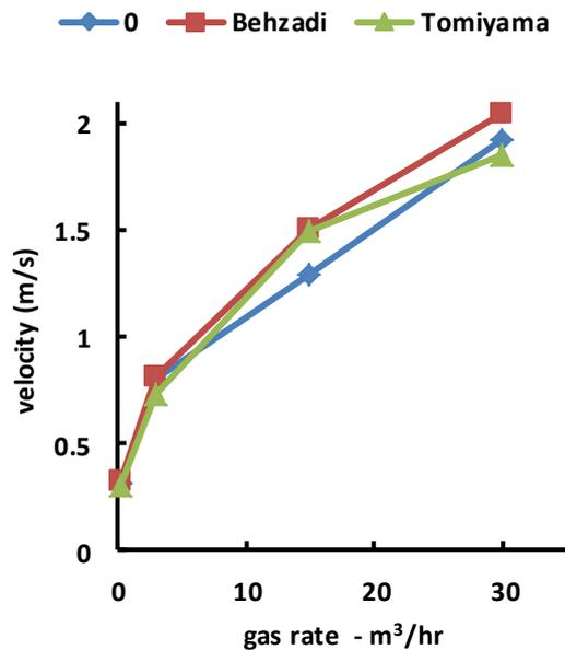
Figure 10: Centre velocity in narrow vessel for different lift expressions as function of gas rate.
