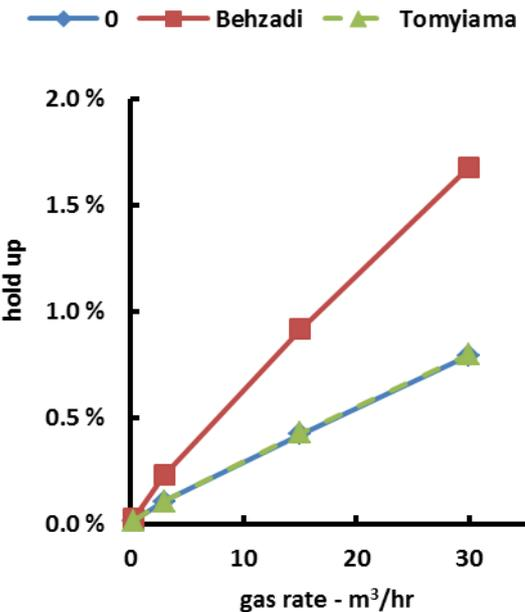
Figure 9: Gas hold up in wide vessel for different lift expressions as function of gas rate.
