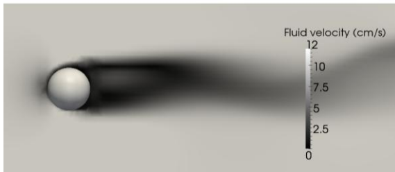
Figure 8: Velocity around a sphere at Re = 300
