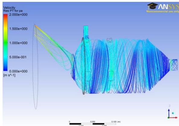
**Figure 8:** Trajectories of the injected particles for gas curtain inlet 3.
