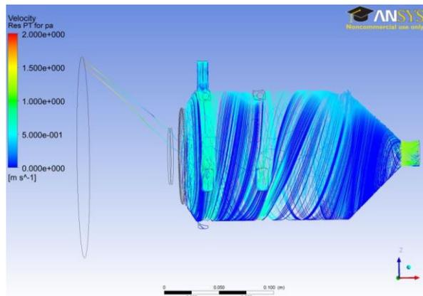
**Figure 7:** Trajectories of the injected particles in gas curtain inlet 2.
