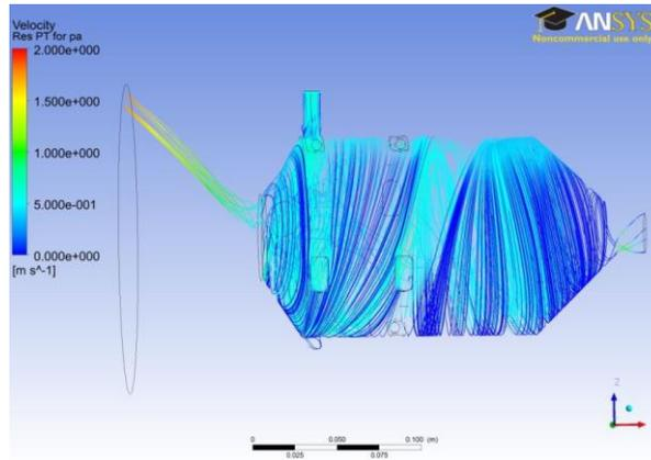
**Figure 6:** Trajectories of the injected particles in gas curtain inlet 1.
