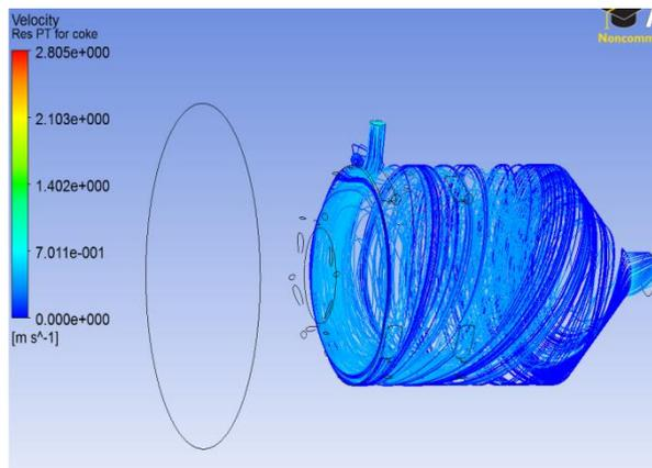
**Figure 11:** Trajectories of the injected particles in Case 6.
