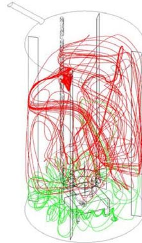
**Figure 8:** PNCr Vessel, Base-case, Acid Streamlines
