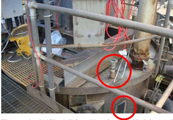
**Figure 6:** PNCr Mixing Vessel – Acid Inlet and Corrosion
