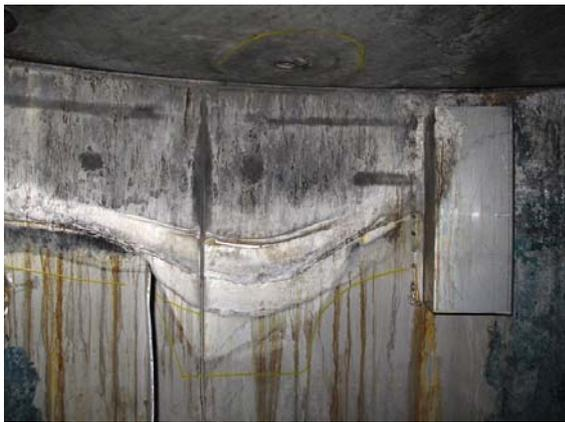
**Figure 7:** PNCr Mixing Vessel – Inner Wall Corrosion
