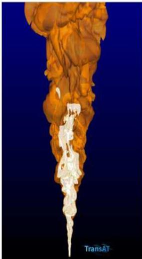
Figure 1: Beginning of gas injection (gas colour is brown; white represents hydrates).
