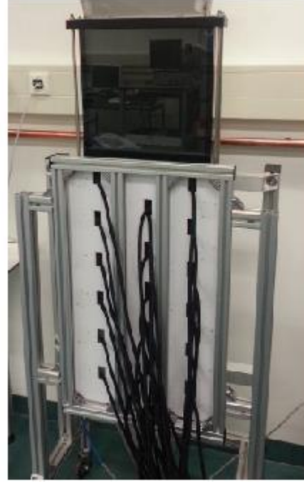
Figure 2: Image of the 2D sensor array in front of the pseudo 2D fluidized bed setup.
