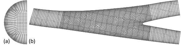
**Figure 4:** Mesh of the arterial geometry, denoting the (a) cross-section mesh of the tubular segments of the geometry, and the (b) hybrid buffer mesh at the bifurcation.
