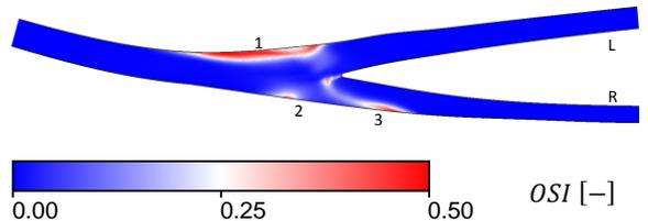
**Figure 9:** Oscillatory shear index contour plot on wall  $\Gamma_{fs}$ .
