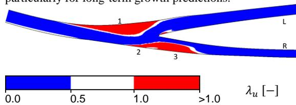
**Figure 10:** Kinetic-energy quotient contour plot of pulsatile perturbations on  $x$ - $y$  symmetry-plane.
