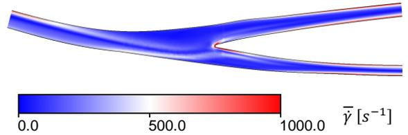
**Figure 8:** Period-averaged strain-rate distribution on  $x$ - $y$  symmetry-plane.
