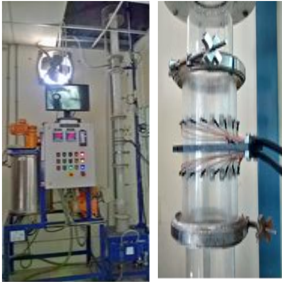
Fig.1 Laboratory column flotation cell
