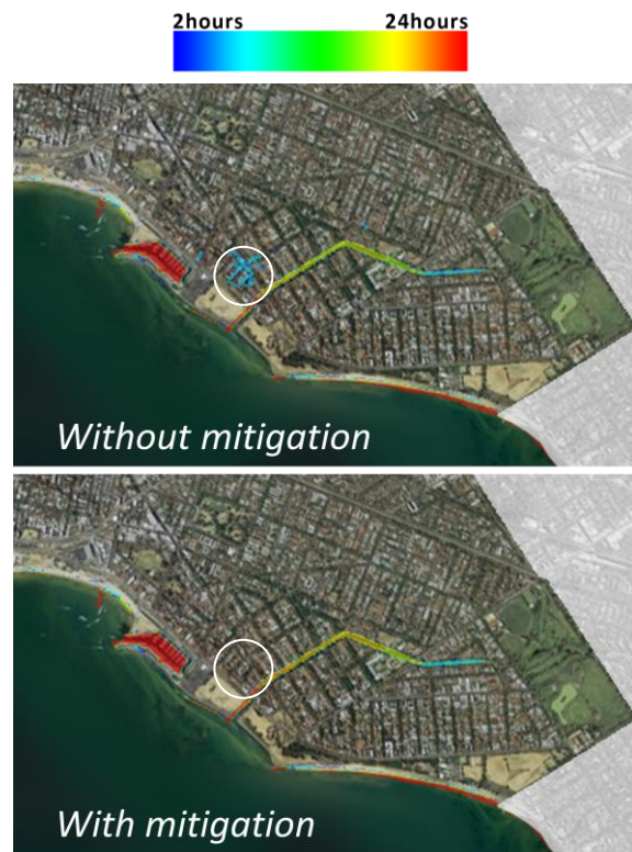
Figure 9: Comparison of the storm-surge flood water retention times in the case of present day sea levels with no rainfall; (a) without mitigation; and (b) with mitigation. The circled region indicates the vicinity of Meredith and Barkly Streets in Elwood.
