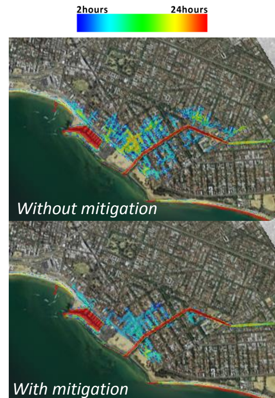
Figure 10: Comparison of the storm-surge flood water retention times in the case of 0.4 m sea level rise with no rainfall; (a) without mitigation; and (b) with mitigation.
