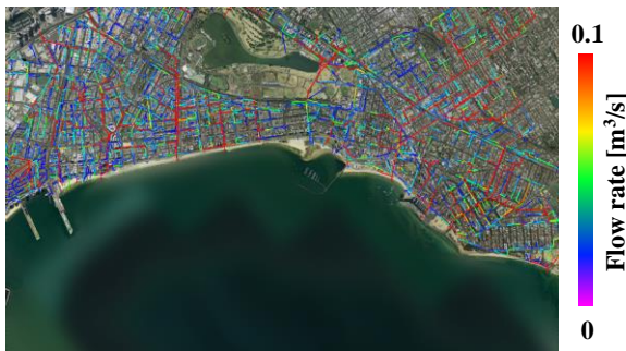
Figure 7: Flow in drainage network for the City of Port Phillip 3 hours after a 1 in a 10 year ARI rainfall.
