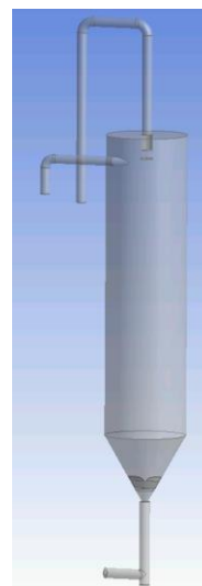
Figure 1: Schematic of modelled domain. Both top and tangential feed lines can be seen. However, only one feed is active at any time. Note, the deflector plate suspended below the top feed nozzle which stops flow from short-circuiting to the outlet.
