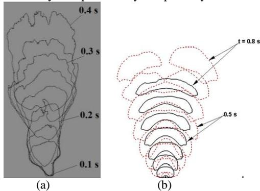
**Figure 11:** Bubble trajectory with time for central injection, (a) experiment for 3.12 m/s (b) CFD predictions for 2 and 3 m/s
