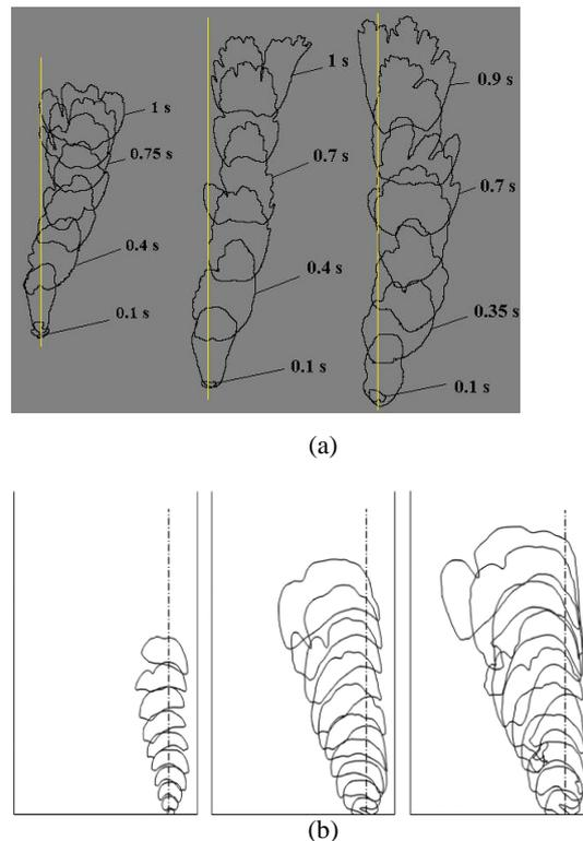
**Figure 12:** Bubble trajectory with time for asymmetric injection, (a) experiments for 1.04 m/s, 2.08 m/s and 3.12 m/s (b) CFD predictions for 80 mm offset at 2, 4 and 6 m/s
