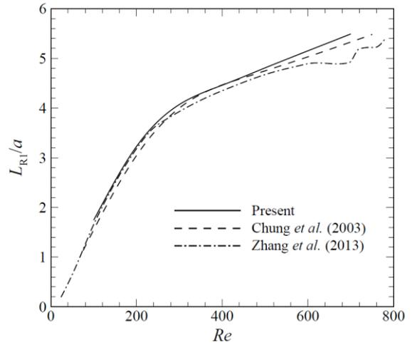
**Figure 5:** Plot of the first recirculation bubble length ( $L_{R1}/a$ ) against Reynolds number ( $Re$ ), comparing the present results to those of Zhang and Poth erat (2013) and Chung *et al.* (2003).
