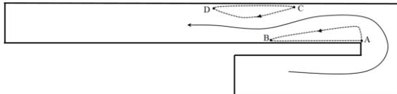
**Figure 4:** Separation (A and C) and reattachment (B and D) points. Reproduced from Zhang and Poth erat (2013).
