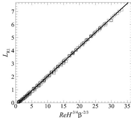
**Figure 14:** Collapse of primary recirculation bubble over ranges of Hartmann  $100 \leq H \leq 500$ ,  $10 \leq Re \leq 2000$  and opening ratio  $0.3 \leq \beta \leq 1$  when plotted against  $ReH^{3/4}\beta^{-2/3}$ . This collapse excludes the regime where the second bubble exists.
