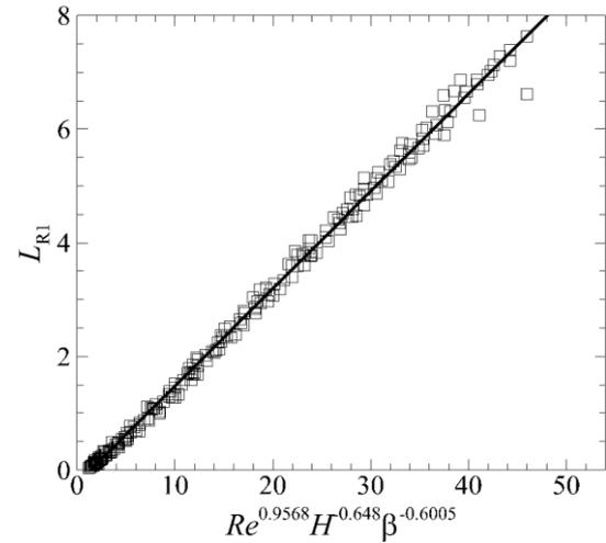
**Figure 13:** Collapse of primary recirculation bubble over ranges of Hartmann  $100 \leq H \leq 500$ ,  $10 \leq Re \leq 3000$  and opening ratio  $0.3 \leq \beta \leq 1$  when plotted against  $Re^{0.9568}H^{-0.648}\beta^{-0.6005}$ .
