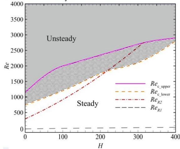
**Figure 7:** Thresholds of Reynolds number where the first bubble and the second bubble start to appear, ( $Re_{R1}$  and  $Re_{R2}$ , respectively) and the flow transitioned from steady to unsteady ( $Re_c$ ) for  $\beta=1$ ,  $0 \leq Re \leq 4000$  and  $0 \leq H \leq 400$ .
