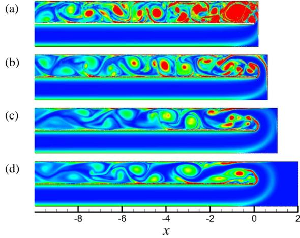
**Figure 10:** The structure of the unsteady flow at  $Re = 1200$  and  $H = 100$  for (a)  $\beta = 0.2$ , (b)  $\beta = 0.5$ , (c)  $\beta = 1$  and (d)  $\beta = 2$  initiated from scratch.
