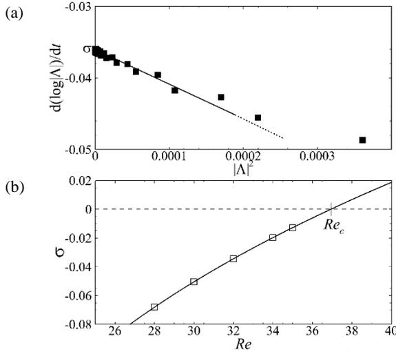
**Figure 3:** Typical plots of (a)  $d(\log|\Lambda|)/dt$  against  $|\Lambda|^2$ , and (b) the infinitesimal growth rate  $\sigma$  against the Reynolds number. The dotted line shows the zero growth rate position, while the solid line shows the fitted function extrapolated to obtain the critical Reynolds number.
