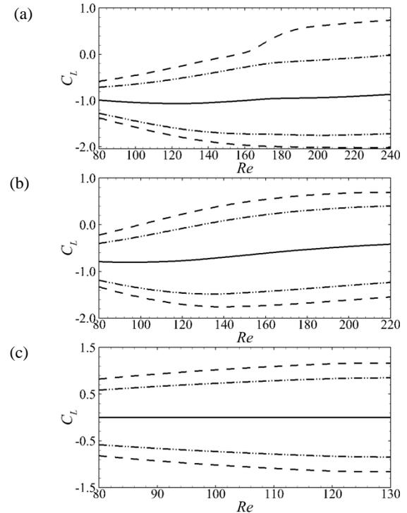
**Figure 9:** Plots of the lift force coefficients against  $Re$  for cylinder inclinations: (a)  $36^\circ$ , (b)  $42^\circ$ , and (c)  $60^\circ$ . The different lines follow the definitions in figure 8.
