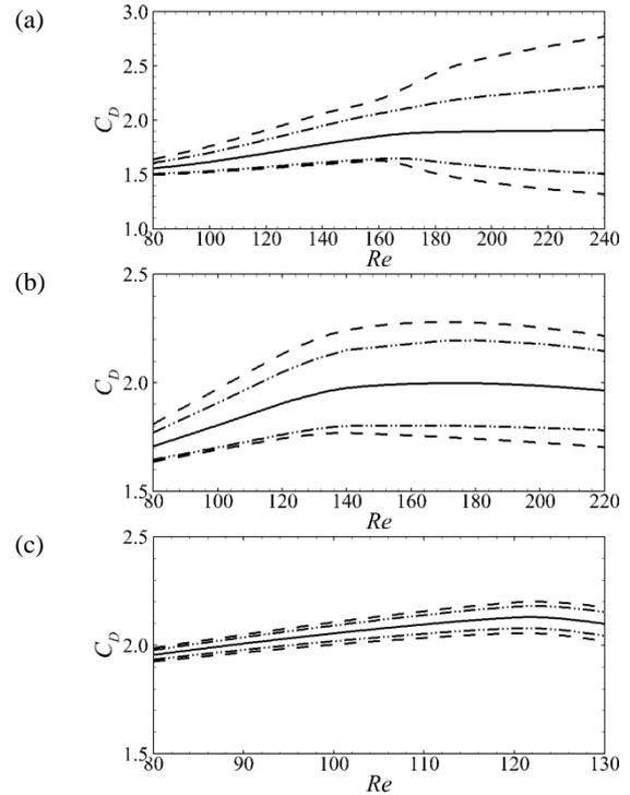
**Figure 8:** Plots of the drag force coefficients against  $Re$  for cylinder inclinations: (a)  $36^\circ$ , (b)  $42^\circ$ , and (c)  $60^\circ$ . Time-averaged force coefficients are given by the solid line, the extrema of the fluctuations by the dashed lines, and the r.m.s. of the fluctuations about the time-averaged value given by the (— · —) line.
