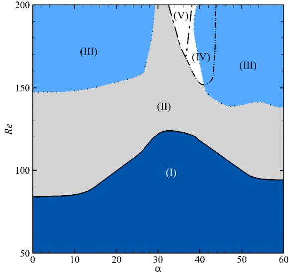
**Figure 5:** Map of the parameter space where the different vortex street shedding modes were observed. (I) is the Kármán vortex street, (II) the bi-layered vortex street, (III) the secondary vortex street, (IV) the P+S-like vortex street, and (V) the 2P-like vortex street. Note region (IV) is bounded within the  $---$ , which intersects with region (III) at higher cylinder inclinations.
