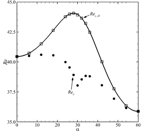
**Figure 4:** Map of the critical Reynolds number  $Re_c$  (●) and  $Re_{c,D}$  (□) as  $\alpha$  is varied. The fitted line is described by equation 3.
