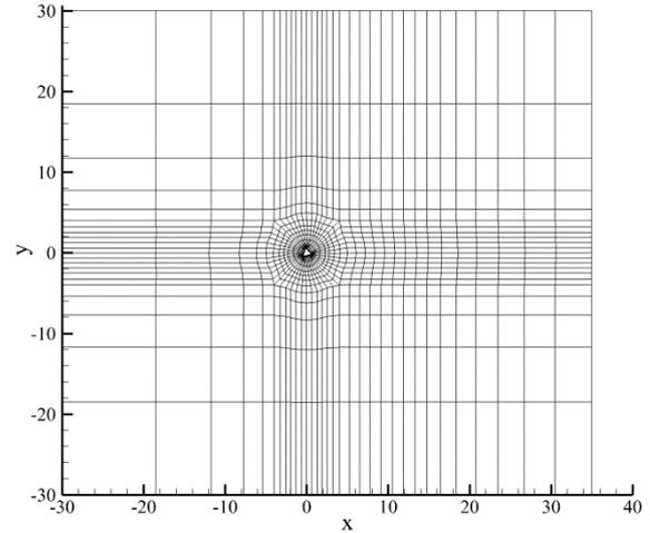
**Figure 2:** Example computational domain utilised for this study showing the macro-element distribution.
