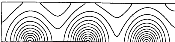
Fig.8. Ion charge density distribution for d_p = 5\mu m & (\rho_p)_{in} = 1g/m^3 ((\rho_{ion})_{max} = 45.3\mu C/m^3, (\rho_{ion})_{max} = 17.1\mu C/m^3, contour interval= 2.01\mu C/m^3 )
