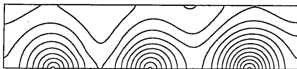
Fig. 5. Ion charge density distribution for d_p = 2\mu m & (\rho_p)_{in} = 1 g/m^3 ((\rho_{ion})_{max} = 37.0\mu C/m^3, (\rho_{ion})_{max} = 11.7\mu C/m^3, contour interval = 1.8\mu C/m^3 )
