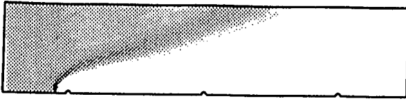
Fig.7. Particle mass concentration for d_p = 5\mu m & (\rho_p)_{in} = 1g/m^3
