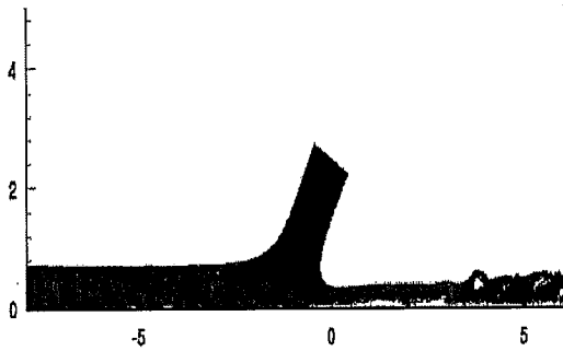
Figure 5. Predicted flow pattern from SPH simulation of an impinging jet onto a moving surface, at Re=800 , plate velocity (right to left) 0.5 times nozzle velocity. \theta = 30 degrees. (Resolution approx 35000 particles).
