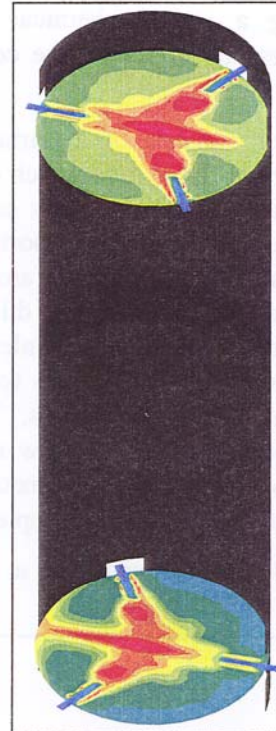
Figure 8: Temperature distribution in cross sections of the HRL pilot-scale gasifier
