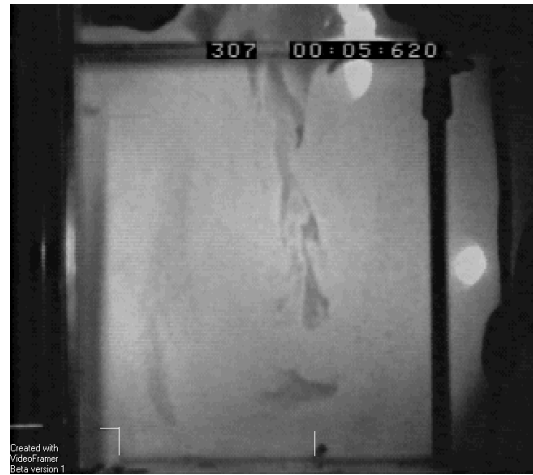
Figure 4: Still photograph of fluidized bed with U_{jet}=327 m/s and U_f=U_{mf} . Uprights represent approximately 0.3m separation. D_o=0.0036 m.
