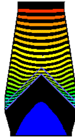
Figure 8: Layered flow pattern with solids consumption and uniform initial burden.
