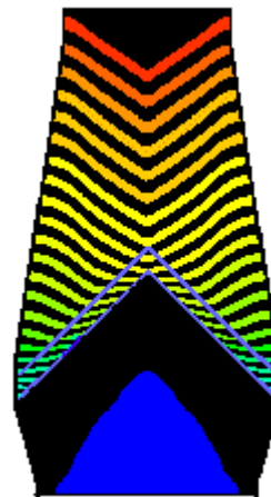
Figure 9: Layered flow pattern with solids consumption and non-uniform initial burden.
