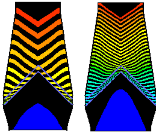
Figure 10. Flow patterns when the overall mass loss rate is: (a) double; and (b) half of that in Fig. 9.
