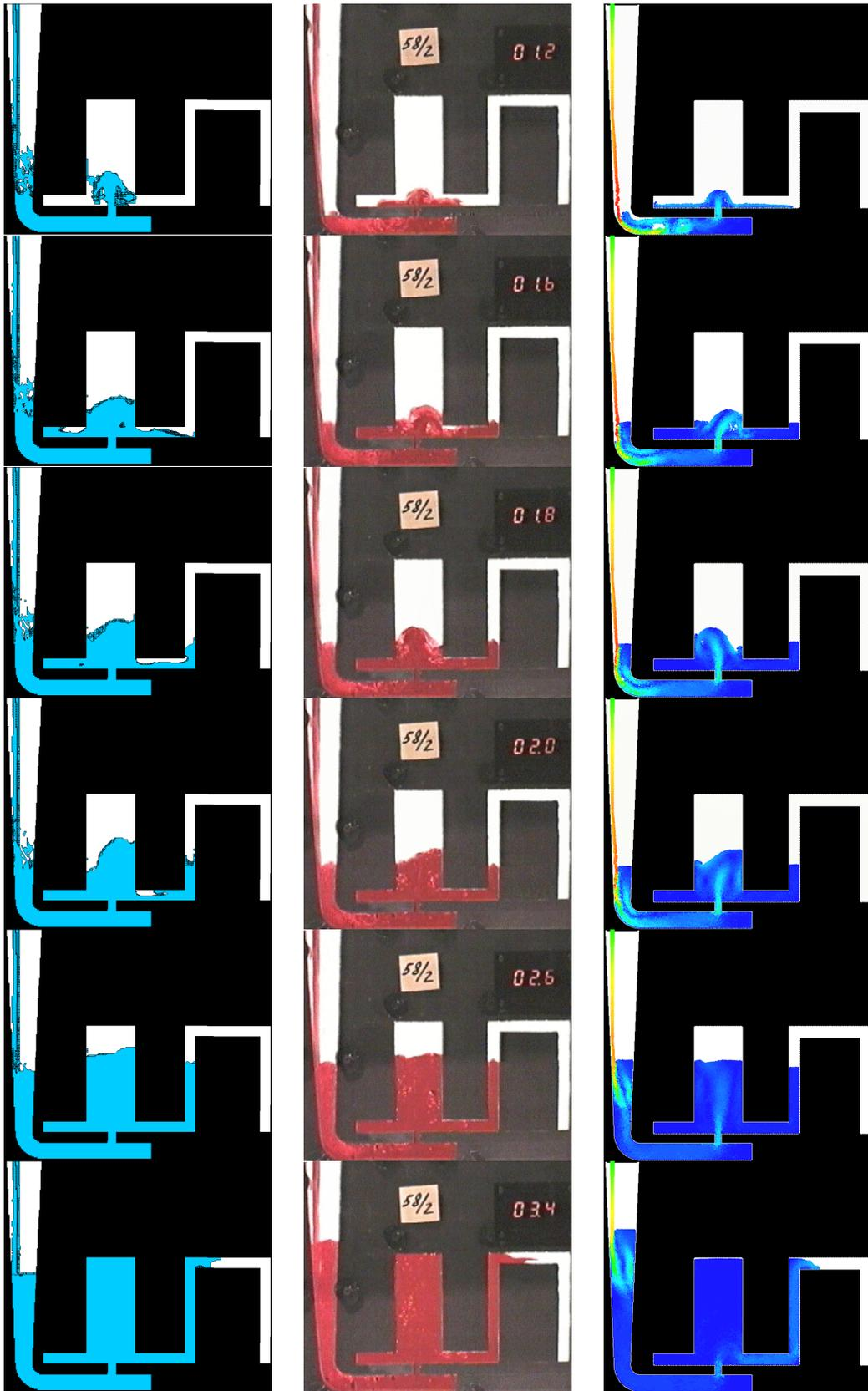
Figure 4: Filling of Model 1. Left: MAGMAsoft. Middle: experiment. Right: SPH.
