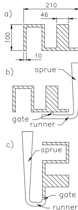
**Figure 1:** Transparent die models. (a) Die cavity geometry. The lengths are in mm and the third dimension is 20 mm thick; (b) Model 1: Bottom gating, single gate; (c) Model 2: Vertical orientation, bottom gating.
