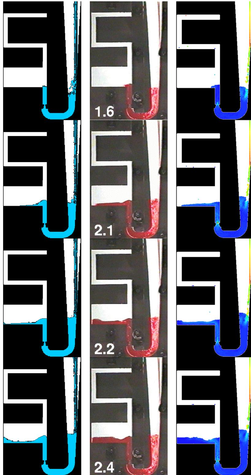
**Figure 5:** Filling of Model 2. Left: MAGMAsoft. Middle: experiment. Right: SPH.
