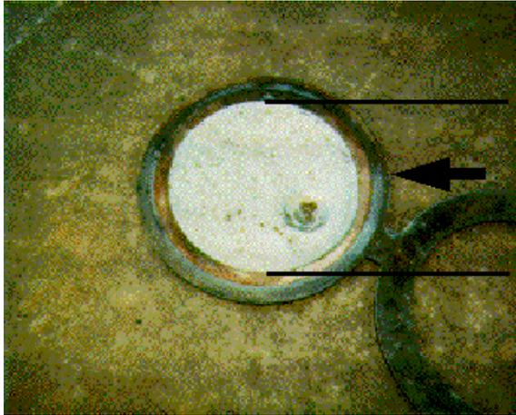
**Figure 2:** Hole in steel blank. Direction of inlet flow to tee-junction is indicated.
