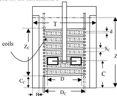
**Figure 1:** Experimental geometry used by Oldshue and Gretton.
