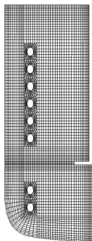
**Figure 2:** Mesh of 5264 control volumes for a proposed geometry.
