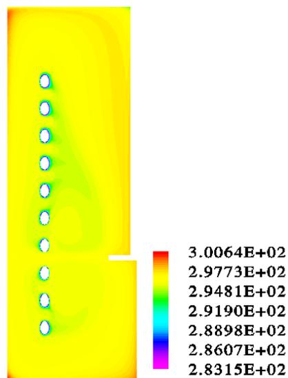
Figure 5: Temperature (K) contour plot for the experimental apparatus.
