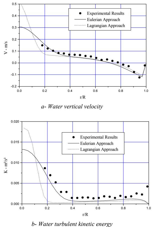
**Figure 10** : Comparison between predicted and experimental data - Wall condition
