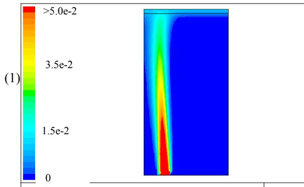
**Figure 6** : Predicted air volume fraction for wall-plume configuration - Eulerian approach.
