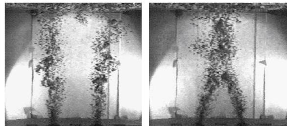
**Figure 3** : 2 plumes configuration at different instants – flow-rate : 5l/min
