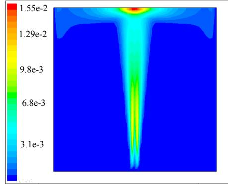
**Figure 7** : Predicted water turbulent kinetic energy for one plume configuration - Lagrangian approach.
