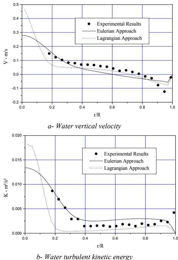
**Figure 9** : Comparison between predicted and experimental data - Symmetry condition.
