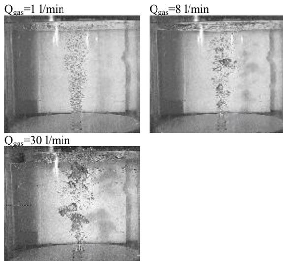
**Figure 1** : Plume behaviour for different air flow-rates.
