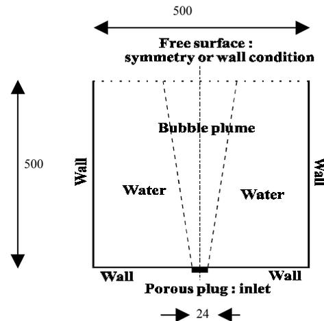
**Figure 8** : Water model characteristics and boundary conditions illustration.
