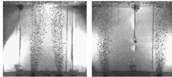
**Figure 2** : 2 plumes configuration at different locations – flow-rate : 1l/min
