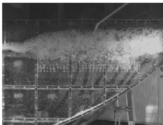
Figure 15a Gas foaming with two CO evolution zones at the flow rate of 164 slpm
