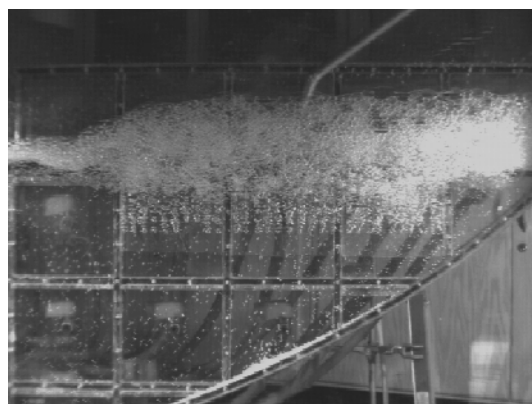
Figure 15a Gas foaming with two CO evolution zones at the flow rate of 164 slpm
