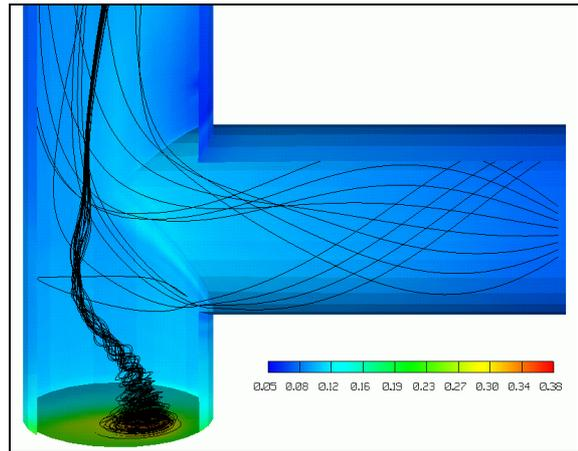
**Figure 5:** Particle concentration (v/v) and fluid phase streamlines. Multi-phase model with swirling inlet flow.
