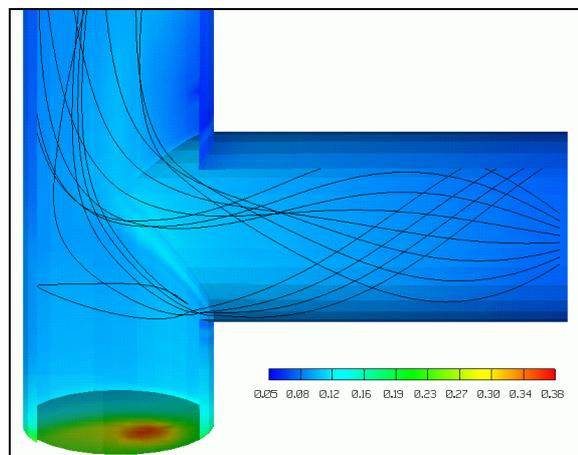
**Figure 6:** Particle concentration (v/v) and fluid phase streamlines (streamlines in blanked end of tee removed for clarity). Multi-phase model with swirling inlet flow.
