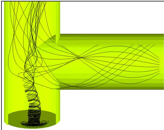
**Figure 7:** Fluid phase streamlines. Single phase model with swirling inlet flow (DSM + Van Leer).
