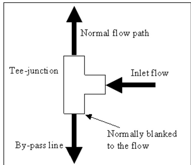
Figure 1: Slurry pipeline tee-junction
