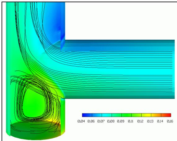
**Figure 4:** Particle concentration (v/v) and fluid phase streamlines. Multi-phase model with uniform inlet flow.
