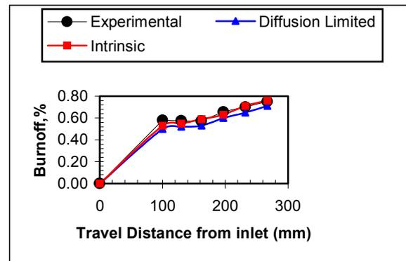
Figure 4: The burn off rate based on different char combustion models
