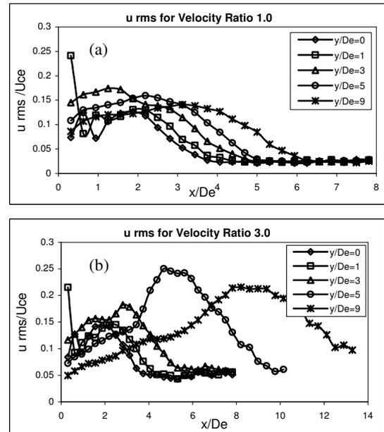
Figure 7(a-b). Comparison of  $u_{rms}$  at the centre of the primary nozzle for jet velocity ratio 1.0 (a) and 3.0 (b)
