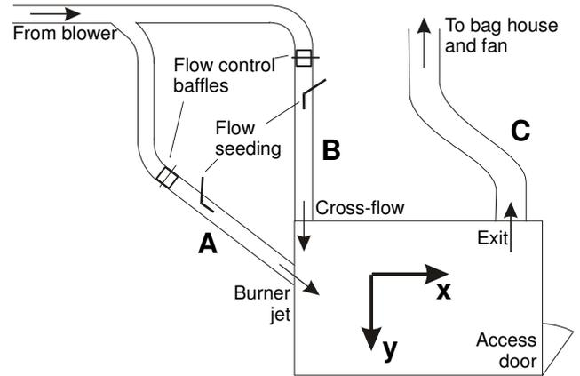
Figure 2. Schematic Diagram of Burner Model and associated ducting
