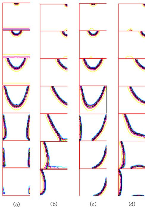
**Figure 7:** GOTHIC Analyses Results of 10 % H<sub>2</sub>/Air Combustion – Hydrogen Mole Fraction ;
