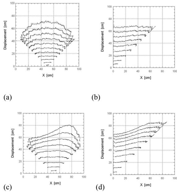
**Figure 5:** Flame Edge Displacement from Ignition Position ;
