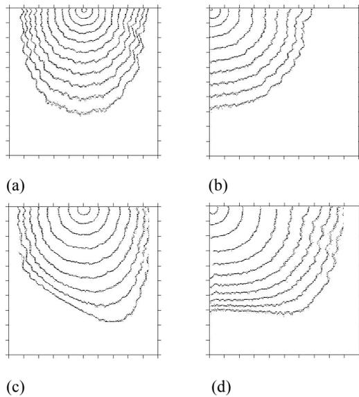
**Figure 4:** Flame Propagation Sequences of 10% H<sub>2</sub>/Air Premixed in 2-D Combustion Chamber ;
