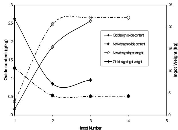
**Figure 5:** Predicted ingot oxide content and weights for the old and new wheel designs at 30 tonnes/hr
