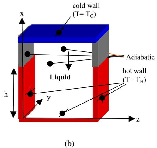
**Figure 1:** Schematic diagram of (a) the physical domain and (b) the simplified configuration studied.
