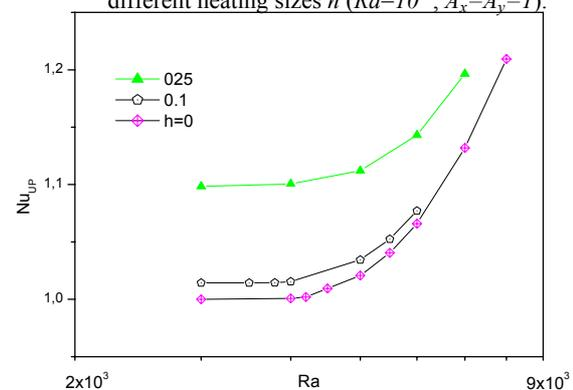
**Figure 3:** Heat transfer as a function of  $Ra$  on the upper surface for different heating sizes  $h$  ( $A_x=A_y=1$ )
