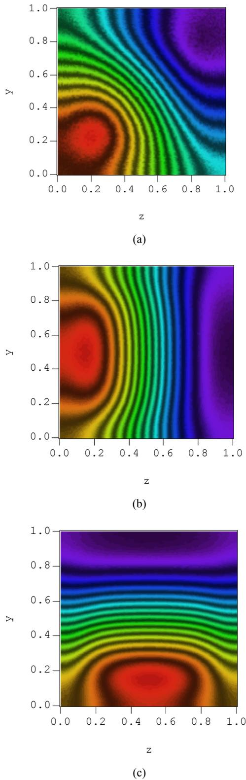
**Figure 4:** The local Nusselt number on the hot-lower surface, for  $h=0$ , at different  $Ra$ , (a)  $4 \times 10^3$ , (b)  $4.5 \times 10^3$  and (c)  $5 \times 10^3$ .
