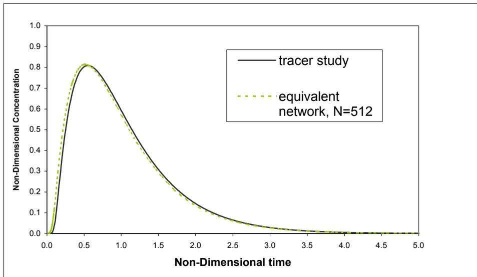
**Figure 5:** Comparison between the tracer study and the network generated from the first set of zones
