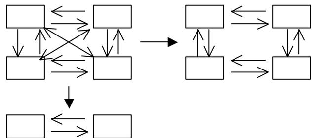
**Figure 2:** main ways of network simplification; (LHS): simplification by lumping cells; (RHS): simplification by reducing number of exchange flows
