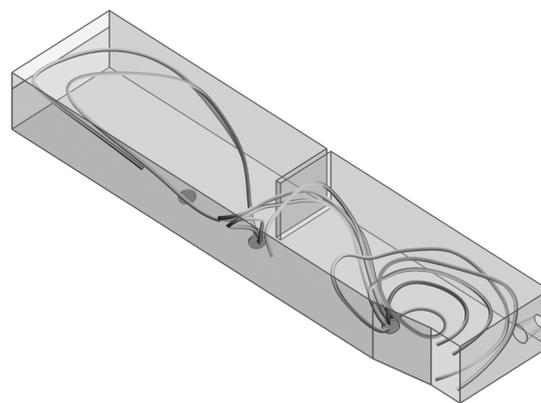
**Figure 4:** Flow-follower paths for four inlet particles (stochastic component removed)
