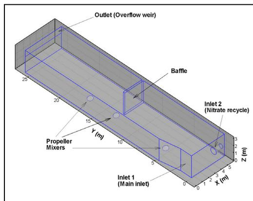
**Figure 3:** Anoxic channel configuration
