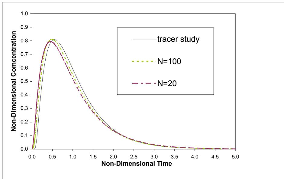
**Figure 6:** RTD comparison between tracer study and different lumping stages
