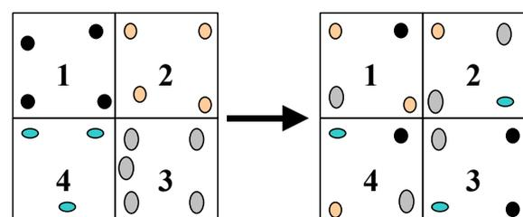
**Figure 1:** Evolution of a closed system during a time step length. The numbers refer to cell number.
