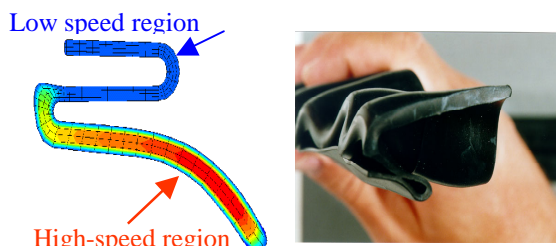
Figure 6a: Initial non-uniform flow distribution through a die result in a highly deformed extruded piece.
