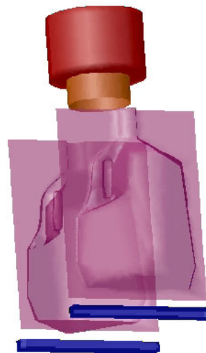
Figure 4: A snapshot of a 3d simulation of blow molding example to make a plastic milk bottle.
