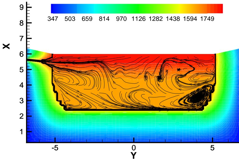
**Figure 4:** Typical temperature distribution (in Kelvin) within iron melt and refractories with molten iron streamlines for variable height coke free layer simulation (dimensions in metres).
