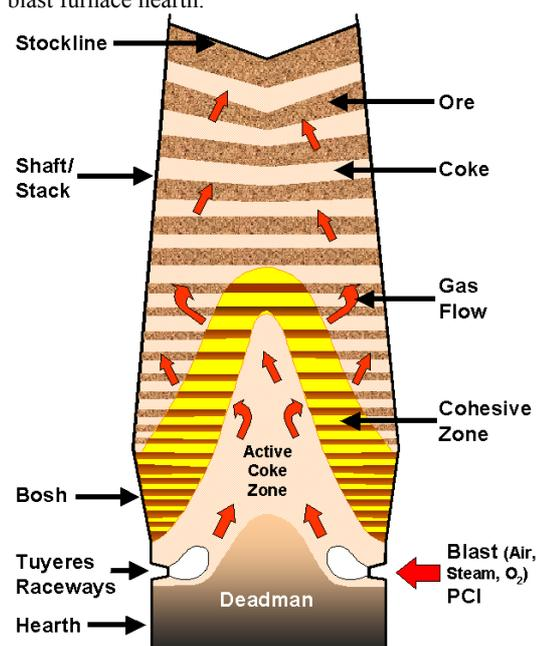
**Figure 1:** The blast furnace process.
