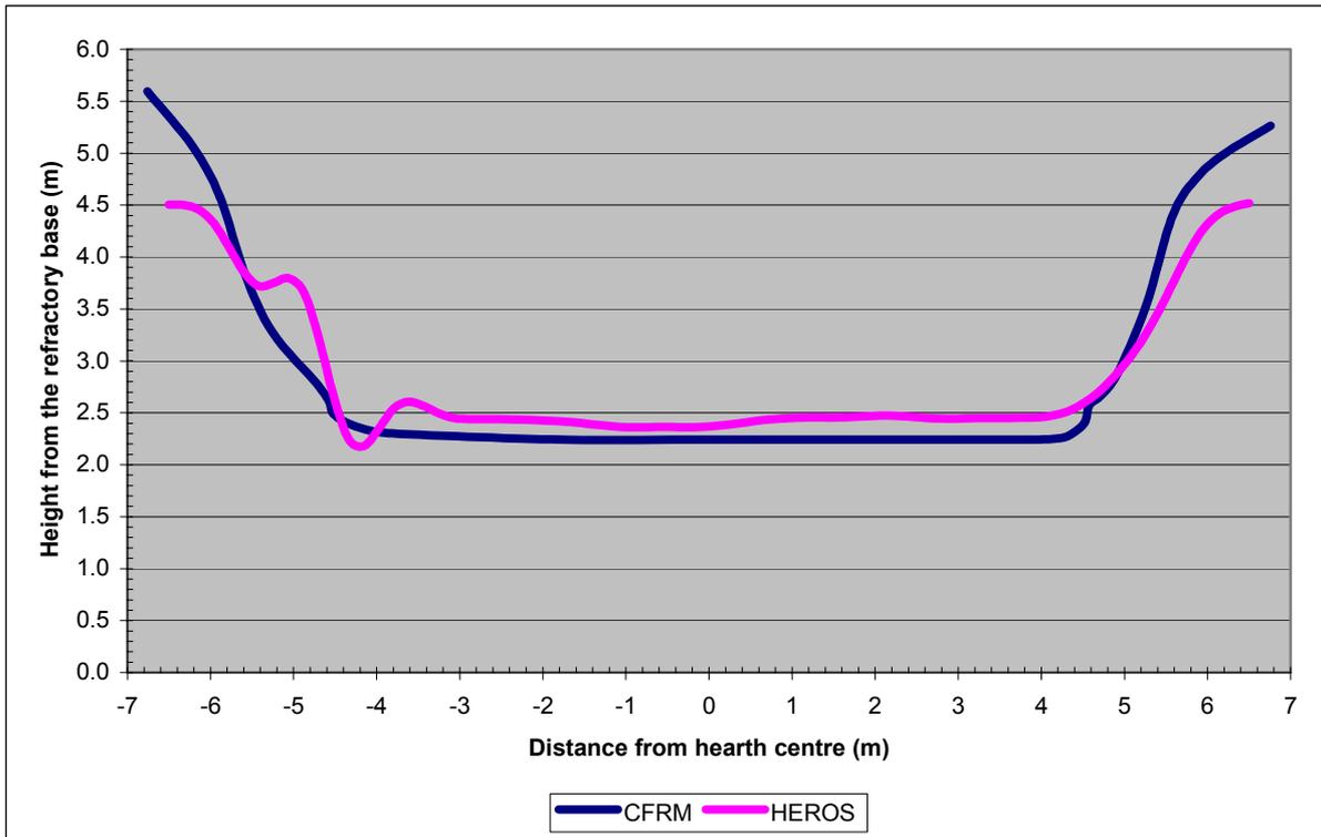
**Figure 8:** Comparison of the position of 1150°C isotherm for CFRM and HEROS model.
