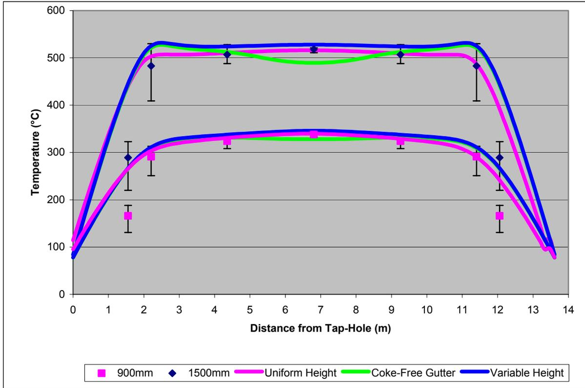
Figure 6: Comparison of pad thermocouple with predictions of CFRM for different CFL shapes.
