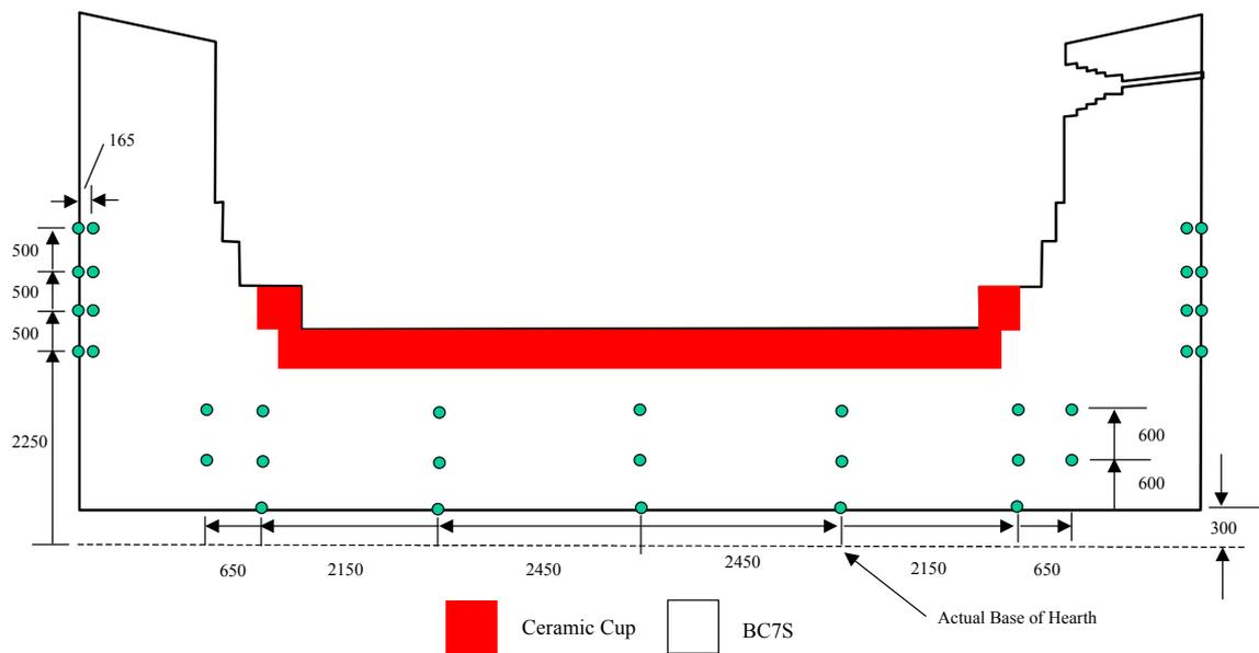
**Figure 5:** Location of thermocouples (green points) in the blast furnace hearth.
