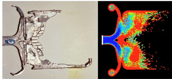
**Figure 12:** Short shot: experiment (left), simulation (right).
