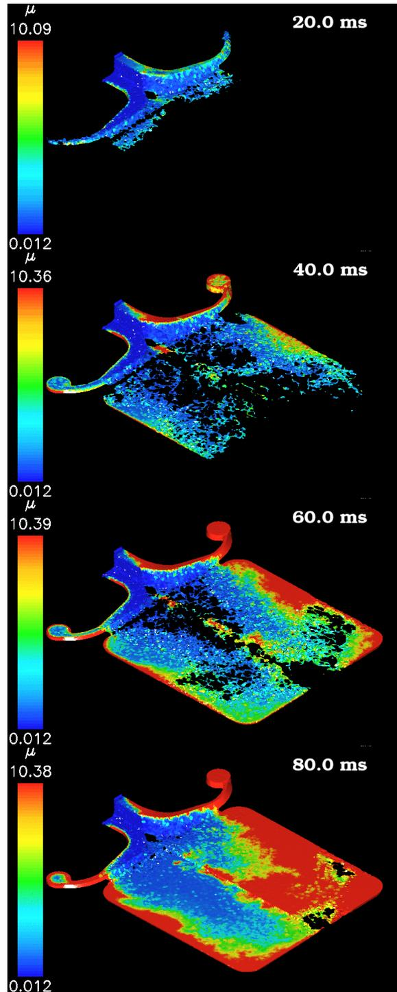
**Figure 11:** Filling of coaster with fluid coloured by viscosity.
