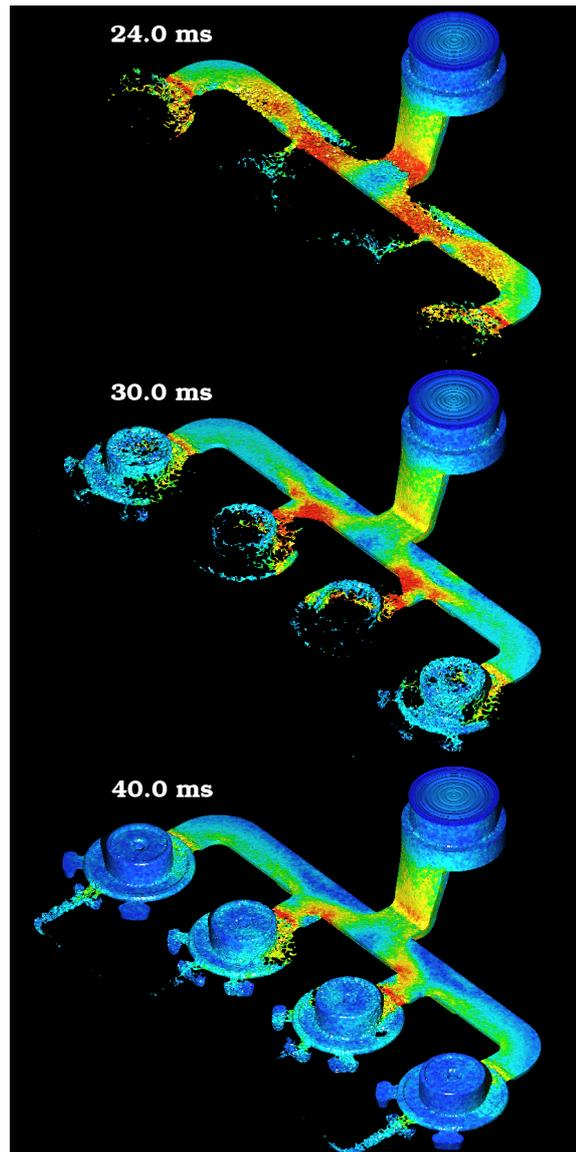
**Figure 2:** Filling of front servo piston at selected times.
