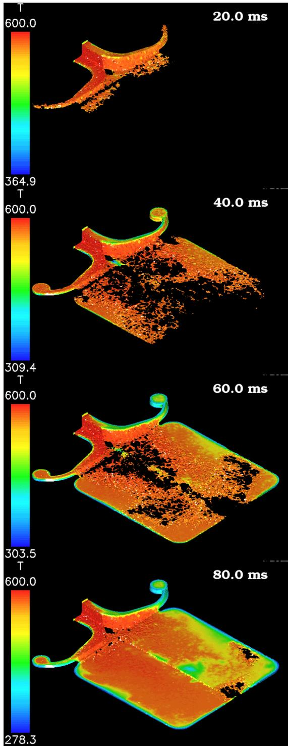
**Figure 10:** Filling of coaster with fluid coloured by temperature.
