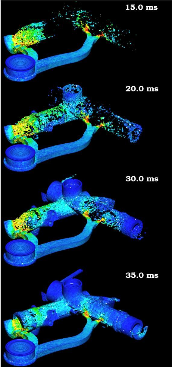
Figure 6: Filling of steering column at selected times.
