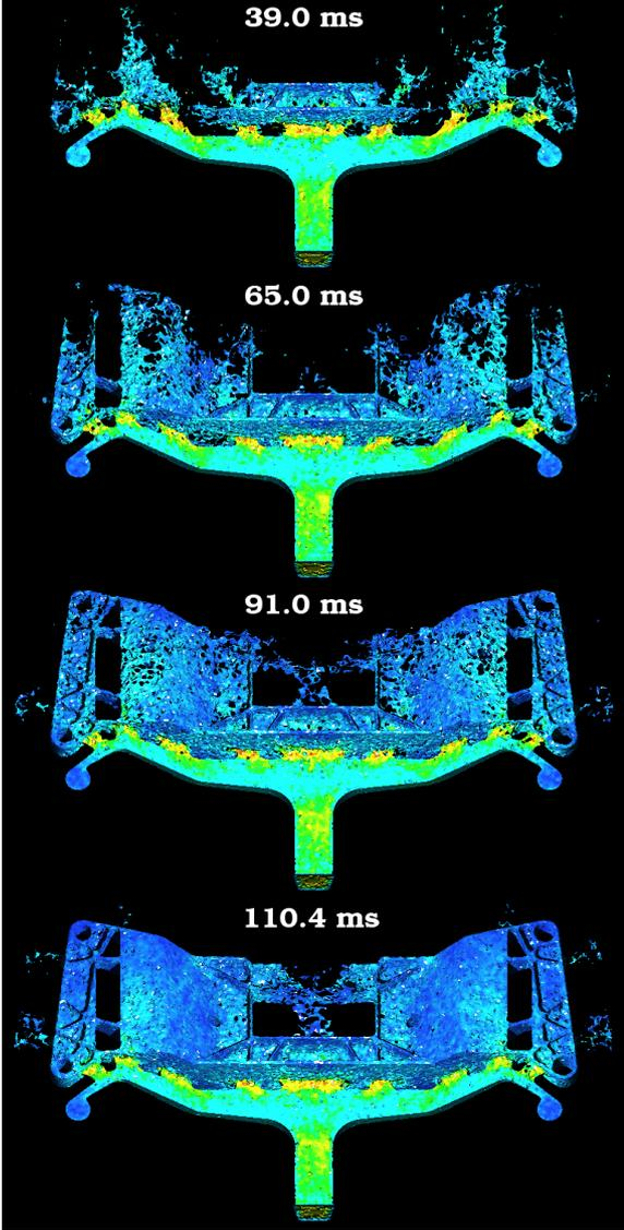
Figure 8: Filling of cross member at selected times.
