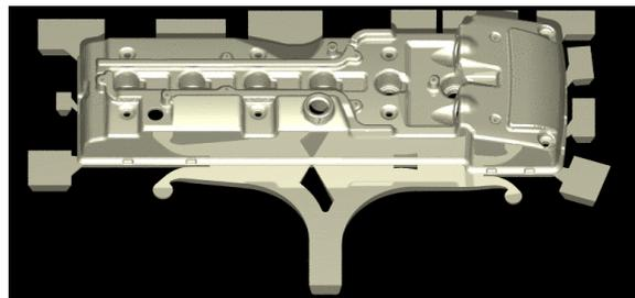
Figure 3: Geometry of rocker cover.
