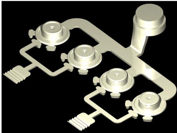
**Figure 1:** Geometry of front servo piston.
