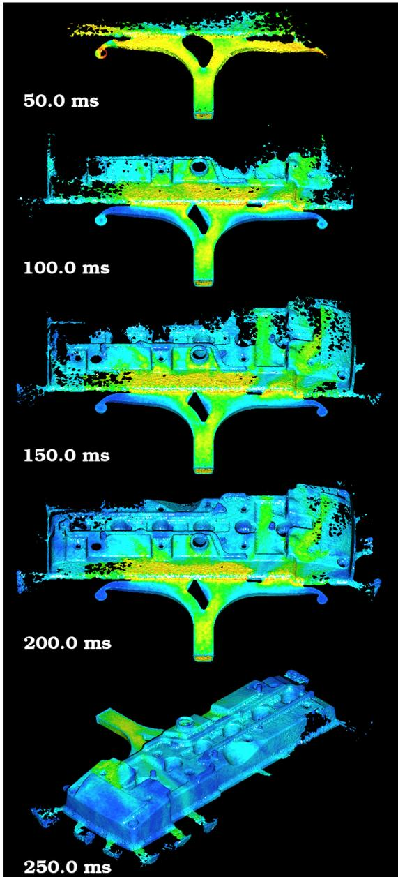
**Figure 4:** Filling of rocker cover at selected times.
