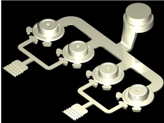
Figure 1: Geometry of front servo piston.
