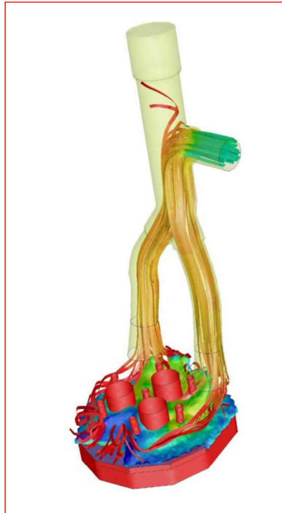
Figure 5 Predicted gas flow in off-gas system at Furnace 1 at Elkem Thamshavn, Norway.
