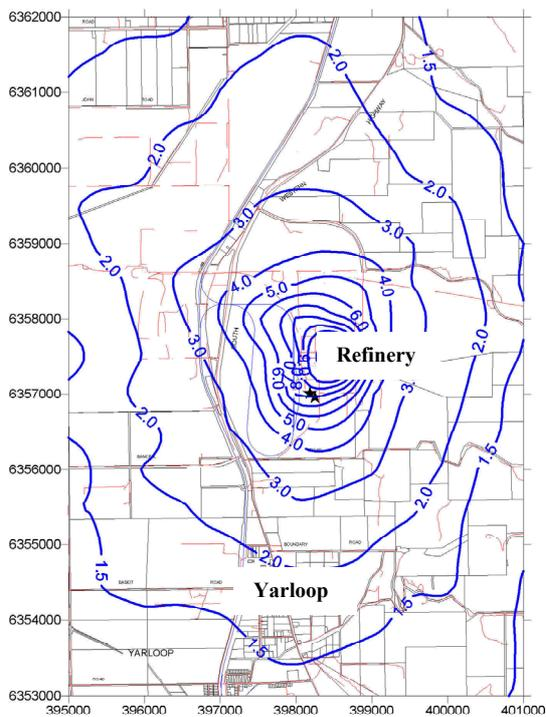
**Figure 18:** Predicted 3-minute, 99.5 percentile ground-level odour values before implementation of 2002 projects
