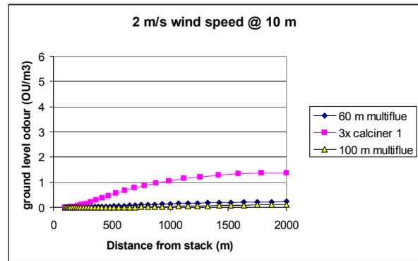
**Figure 9:** Ground-level odour with 2 m/s wind.
