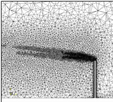
**Figure 3:** CFX-5 mesh after mesh adaption using odour concentration gradients.
