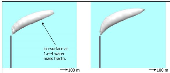
**Figure 8:** Calciner 4 visible plume with no ambient air addition (left) and with 200 TPH ambient air addition (right) at 15 °C.
