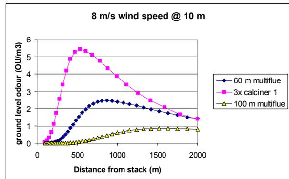
**Figure 11:** Ground-level odour with 8 m/s wind.
