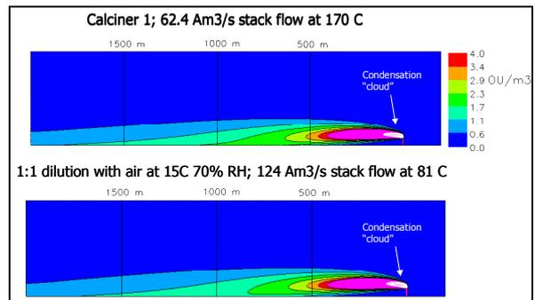
**Figure 6:** Odour contours and plume visibility for ambient air addition to calciner 1 (CFX-4 model).
