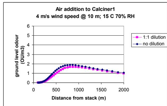
**Figure 7:** Ground-level odour variation for ambient air addition to calciner 1 (CFX-4 model).
