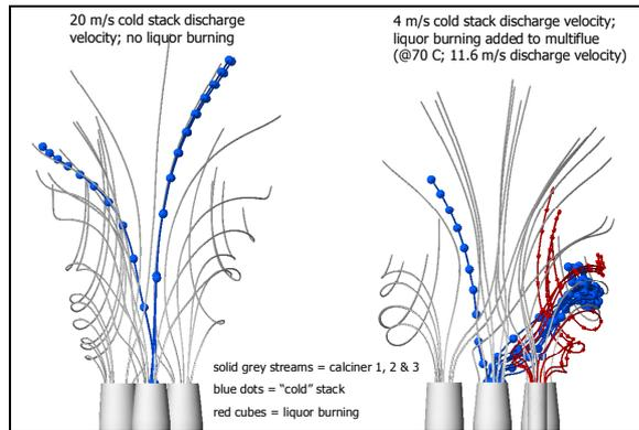
**Figure 14:** Initial plume mixing for cases 1 & 2.
