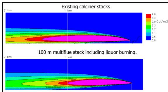
**Figure 17:** Odour contours for current and multiflue stacks to 2 km (CFX-5 models).
