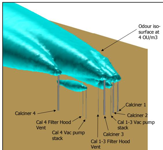
**Figure 12:** Layout of existing stacks (CFX-5 model).
