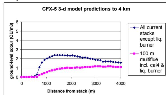
**Figure 16:** Ground-level odour for current and multiflue stacks.
