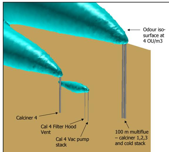
**Figure 13:** Layout of multiflue stack (CFX-5 model)
