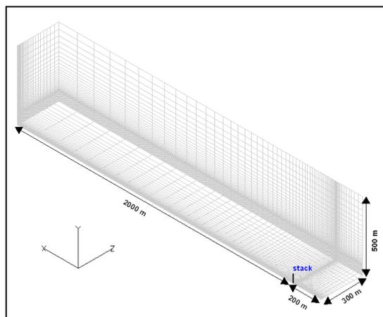
**Figure 1:** Computational domain for plume visibility calculations (CFX-4).
