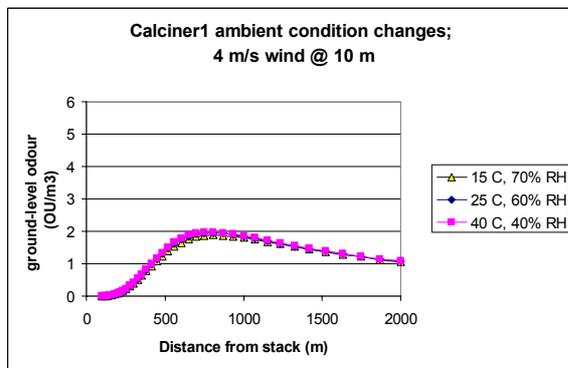
**Figure 5:** Ground-level odour variation with different atmospheric conditions (CFX-4 model).
