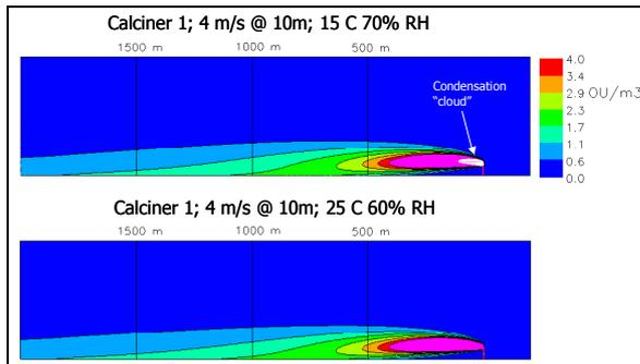
**Figure 4:** Odour contours and plume visibility for two atmospheric conditions (CFX-4 model).
