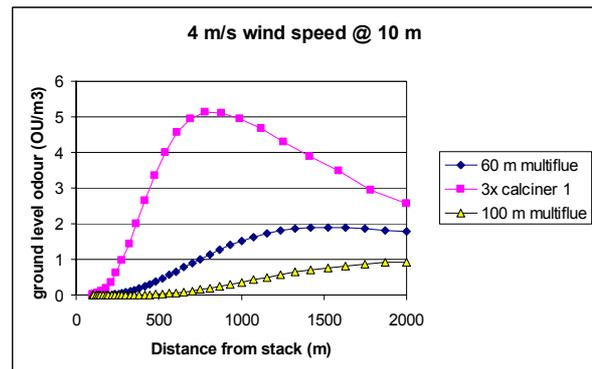
**Figure 10:** Ground-level odour with 4 m/s wind.
