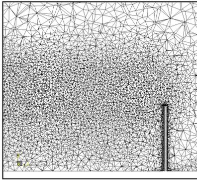
**Figure 2:** CFX-5 mesh prior to mesh adaption.
