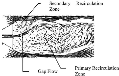
**Figure 2.** Coherent structure in flow over a slitty bluff body
