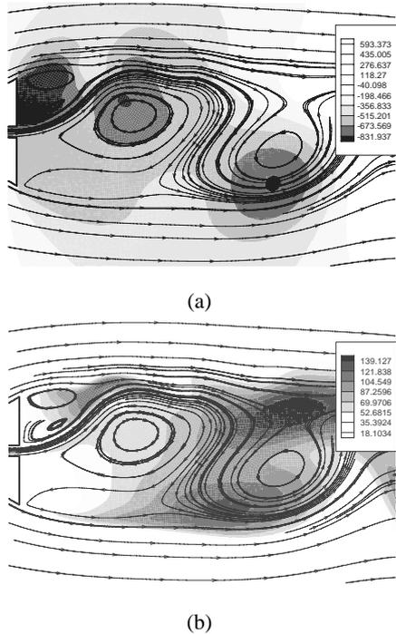
**Figure 5.** Instantaneous character of the near wake (a) static pressure (b) turbulent kinetic energy
