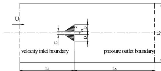
**Figure 1:** Definition of the co-ordinate and the geometrical parameters for the flow past a slitty bluff body
