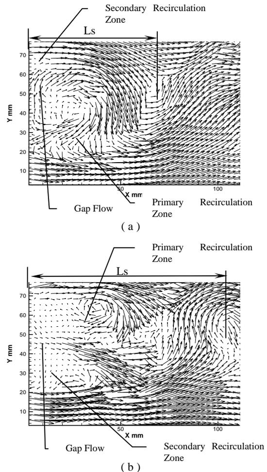
**Figure 6.** Instantaneous vectors of (a) ( $G/D=0$ ) and (b) ( $G/D=0.22$ ) by PIV
