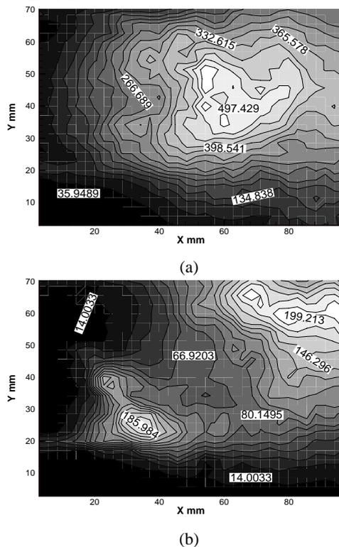
**Figure 8.** Turbulent kinetic energy contour by PIV (a)  $G/D=0$  (b)  $G/D=0.22$
