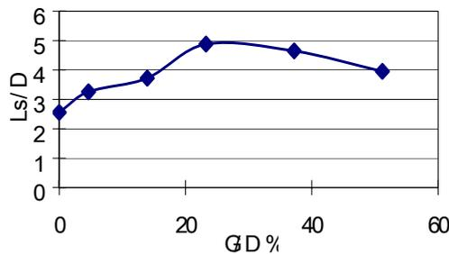
**Figure 7.** Effect of gap ratio on change of vortex shedding character dimension
