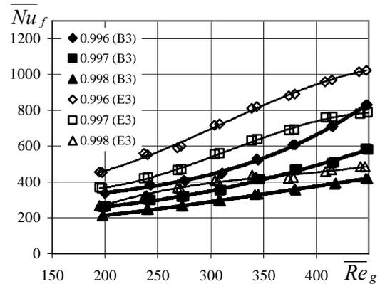
**Figure 5:** Heat transfer of the third tube for upward (B3) and downward (E3) foam flow;  $\beta=0.996$ , 0.997 and 0.998
