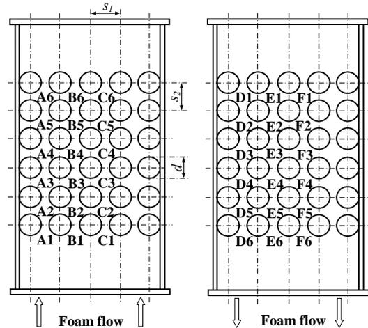
**Figure 2:** The in-line tube bundle in upward and downward foam flow
