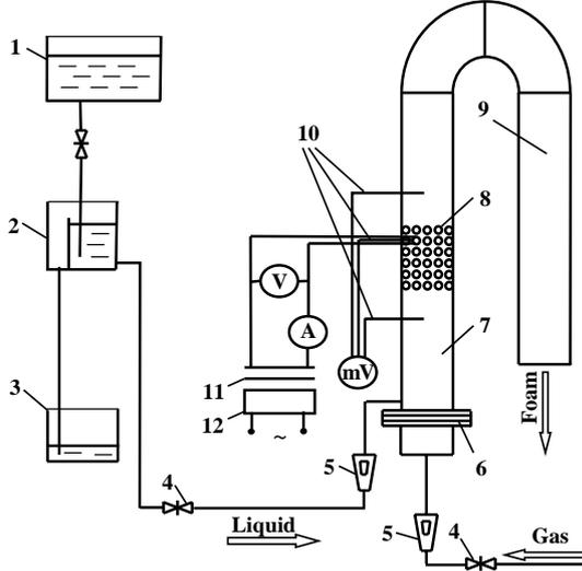
**Figure 1:** Experimental set-up scheme: 1–liquid reservoir; 2–liquid level control reservoir; 3–liquid receiver; 4–gas and liquid control valves; 5–flow meter; 6–foam generation riddle; 7–experimental channel; 8–tube bundle; 9–output channel; 10–thermocouples; 11–transformer; 12–stabilizer
