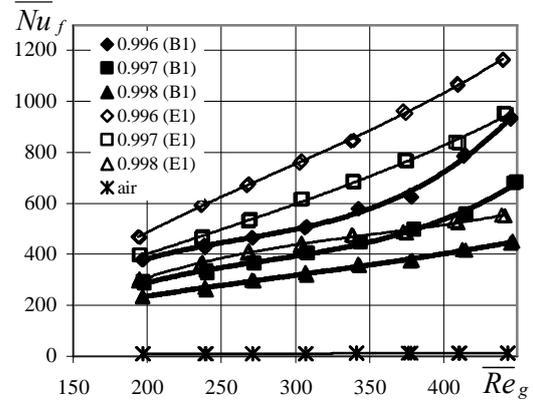
**Figure 4:** Heat transfer of the first tube for upward (B1) and downward (E1) foam flow;  $\beta=0.996$ , 0.997 and 0.998; and the heat transfer of the tube B1 in airflow
