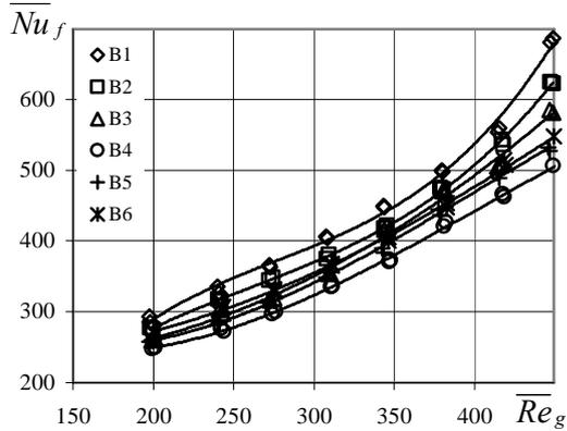
**Figure 6:** Heat transfer intensity of the tubes in the middle-line in upward foam flow,  $\beta=0.997$
