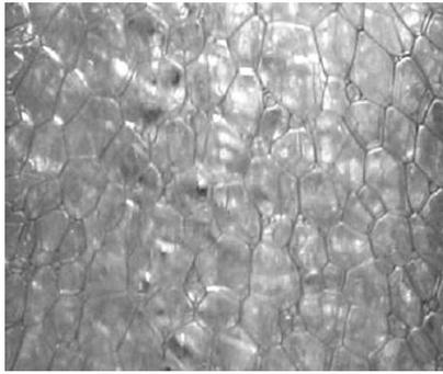
**Figure 3:** Statically stable foam flow in the experimental channel
