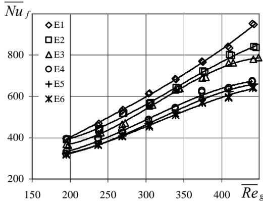
**Figure 7:** Heat transfer intensity of the tubes in the middle-line in downward foam flow,  $\beta=0.997$
