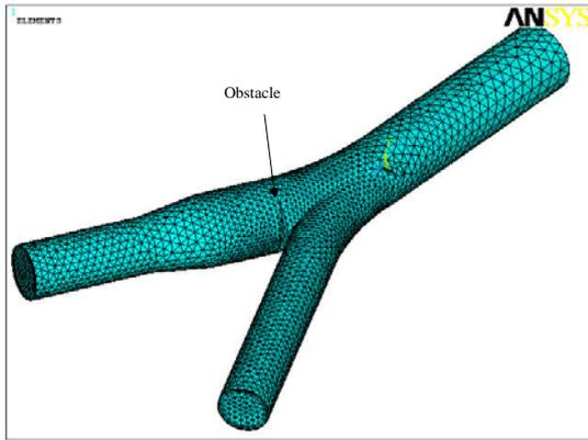
**Figure 4:** Computational mesh used in the CFD study.
