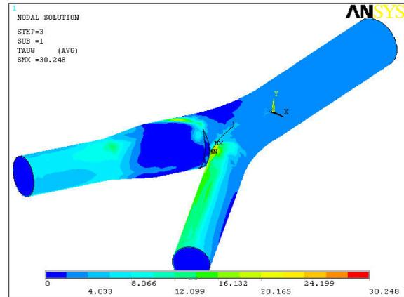
**Figure 7:** Distribution of the wall shear stress.
