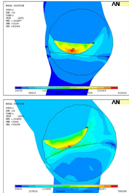
Figure 10. Von-Mises stress in the obstacle.
