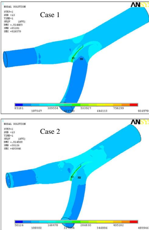
Figure 9. Von-Mises stress in the outer layer.
