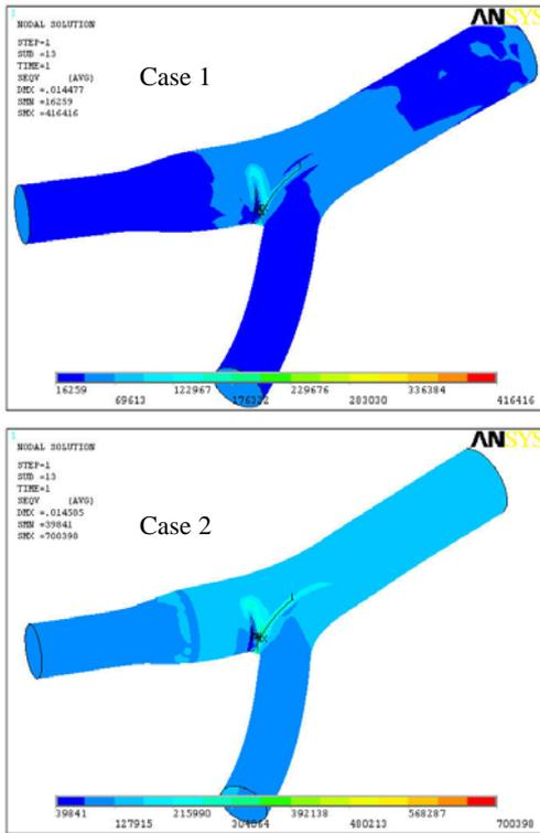
Figure 8: Von-Mises stress<sup>1</sup> in the inner layer.
