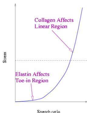
**Figure 3:** Typical structural behaviour of a blood vessel.
