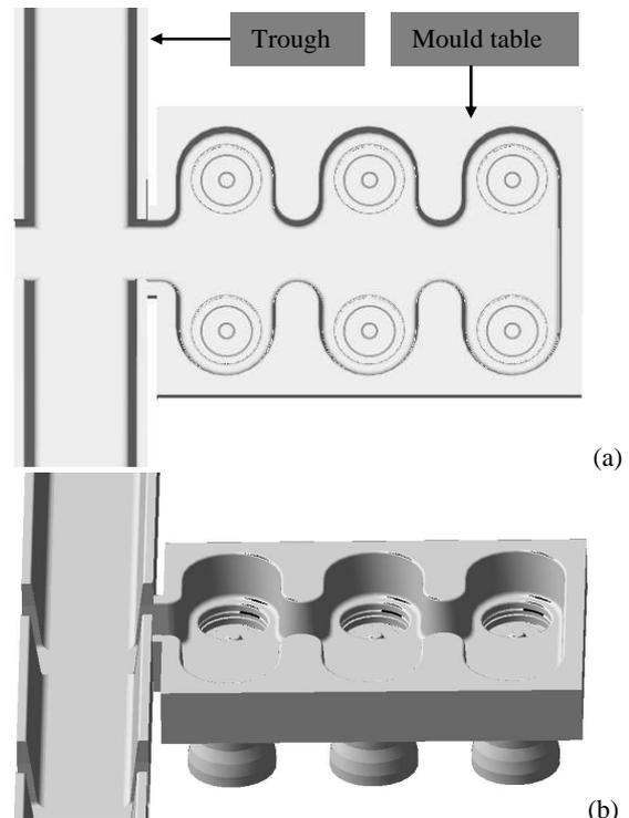
**Figure 1:** Schematic showing (a) a vertical and (b) a side view of the DC Casting configuration with a trough and mould table containing six moulds.
