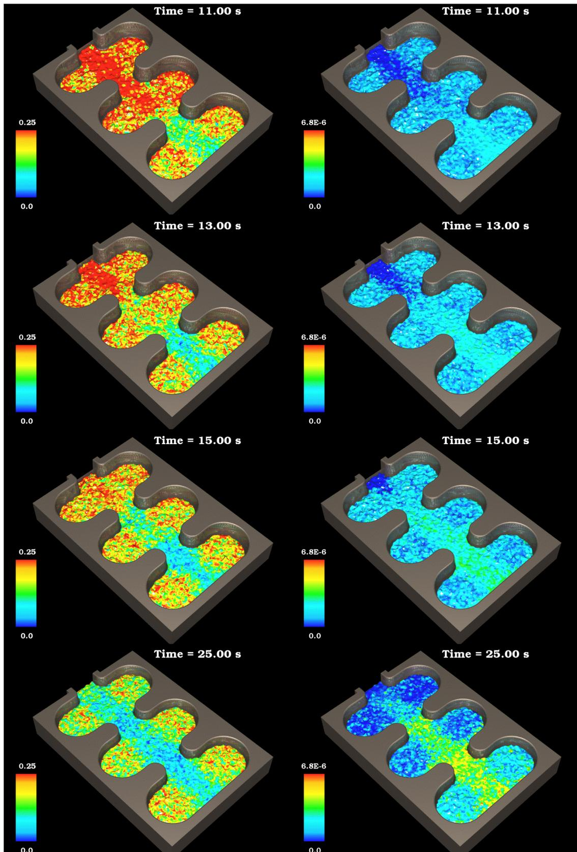
**Figure 4:** Filling patterns of DC mould table at different times. The fluid is coloured by speed (left column) and by oxide mass (right column).
