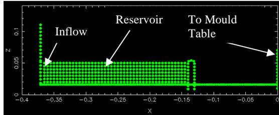
**Figure 2:** Cross section of the constant head inflow reservoir used to control the inflow to the mould table.
