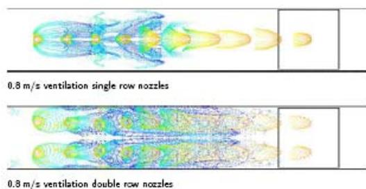
**Figure 8:** Distribution of mist in the tunnel 5s after activation for a ventilation velocity of 0.8 m/s
