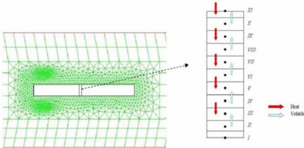
**Figure 2:** The airflow and belt domain discretisation schemes
