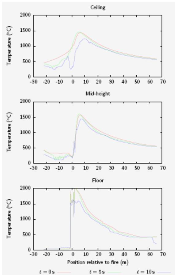
**Figure 7:** Reduction of temperature with time for a ventilation velocity of 0.8 m/s with single row of nozzles at 1.5 m spacing
