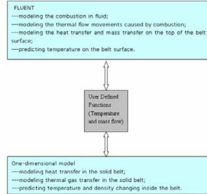
**Figure 3:** The coupling of data exchange between the two models using a UDF
