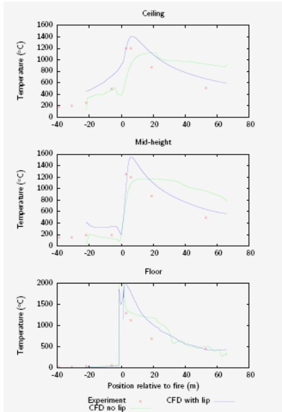
**Figure 5:** Comparison between CFD predictions and data with a ventilation velocity of 0.8 m/s
