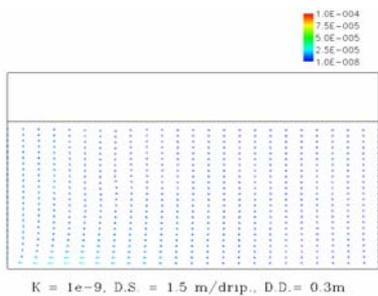
**Figure 5:** Flow field (m/s) for  $K = 10^{-9}\text{ m}^2$
