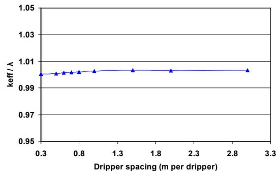
**Figure 2:** Effect of dripper spacing on heat transfer enhancement,  $H = 0.3\text{m}$ ,  $K = 10^{-10} \text{ m}^2$
