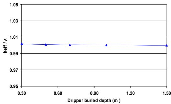
**Figure 3:** Effect of dripper buried depth on heat transfer enhancement,  $b = 0.7\text{m/dripper}$ ,  $K = 10^{-10}\text{ m}^2$
