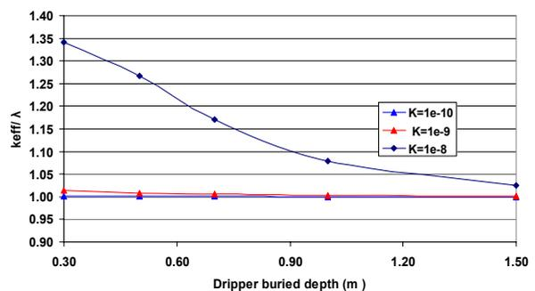
**Figure 8:** Effect of dripper buried depth on heat transfer enhancement for various  $K$ ,  $b = 0.7\text{ m / dripper}$
