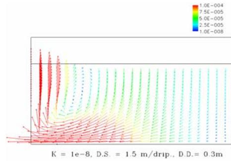
**Figure 6:** Flow field (m/s) for  $K = 1e-8\text{ m}^2$
