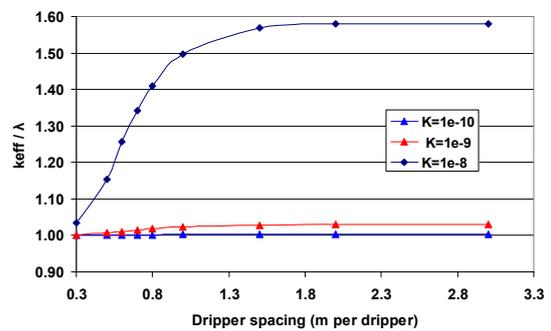
**Figure 7:** Effect of dripper spacing on heat transfer enhancement for various  $K$ ,  $H = 0.3\text{m}$
