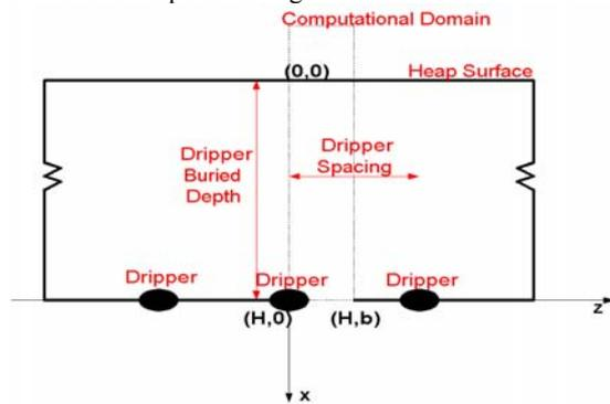
**Figure 1:** Schematic Heap Dripper Zone
