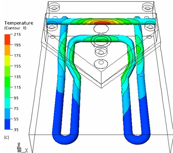
**Figure 4:** Contour Plot of Water Passage Wall Temperature in the Model for the Original Breast Plate Design Scenario.
