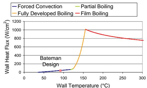
**Figure 6:** Nukiyama Boiling Curve for 50mm diameter, 0.1MPa, 1.8m/s, 35°C supply
