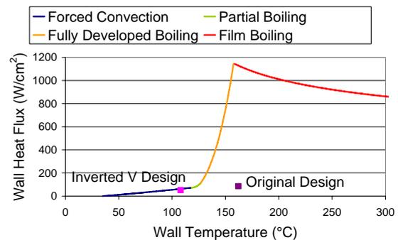
**Figure 5:** Nukiyama Boiling Curve 32mm diameter, 0.1MPa, 1.8m/s, 35°C supply
