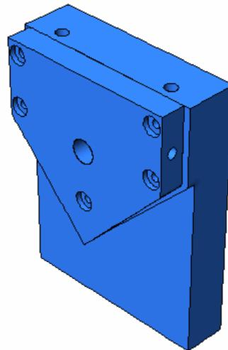
**Figure 2:** Geometry of copper coolers. Original breast plate in foreground, tapping block behind.
