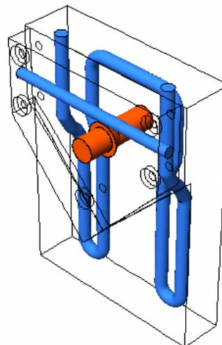
**Figure 3:** View of geometry showing internal detail for the original breast plate case. Water passages shown in blue, tapping channel shown in red. Note funnel shaped wear profile at cold face of rear tapping block.
