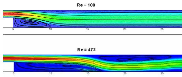
**Figure 2a.** Stream traces for the different Reynolds number (Number of elements =14847, Nodes =7876)
