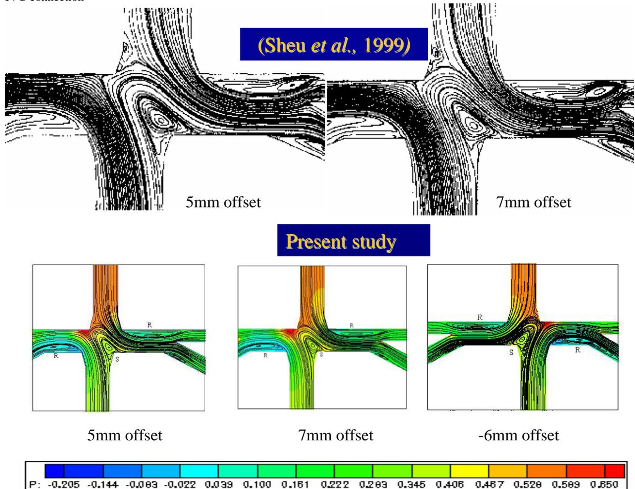
**Figure. 3b** Flow pattern with stream traces in Cavopulmonary connection for the offset 5mm, 7mm and -6mm offsets. S-Stagnation point, R-Re-circulation.
