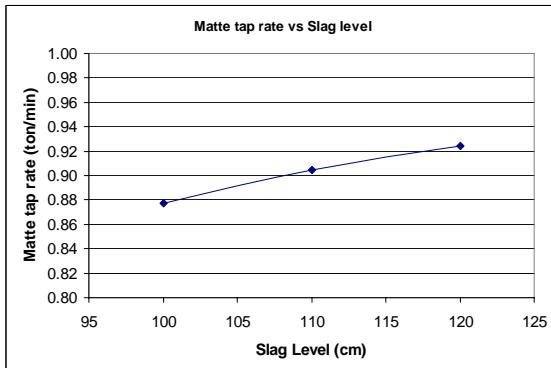
**Figure 12:** Matte tapping rate vs Slag level. Matte level - 65cm, Matte temperature - 1450°C, Slag temperature - 1650°C.
