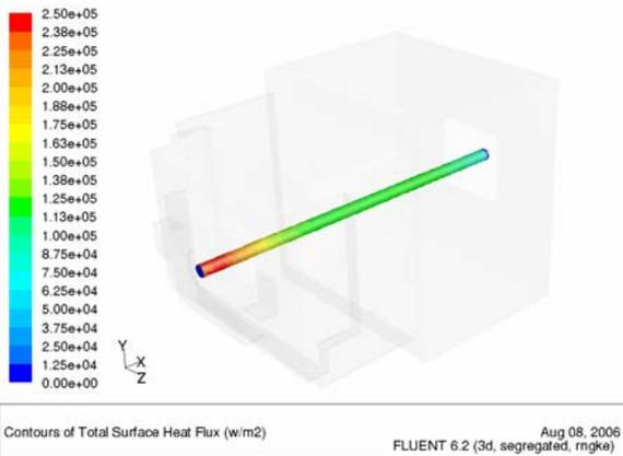
**Figure 5:** Heat flux distribution from the matte. Largest heat fluxes occurring around the front of the tap channel where the copper is closer to the matte.
