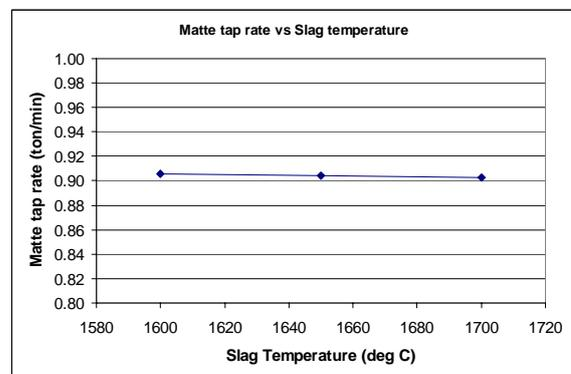
**Figure 10:** Matte tapping rate vs Slag temperature. Matte level – 65cm, Slag level - 110cm, Matte temperature - 1450°C
