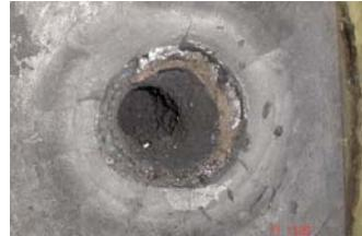
**Figure 3:** Graphite brick during the second and third test showing a very enlarged tap hole
