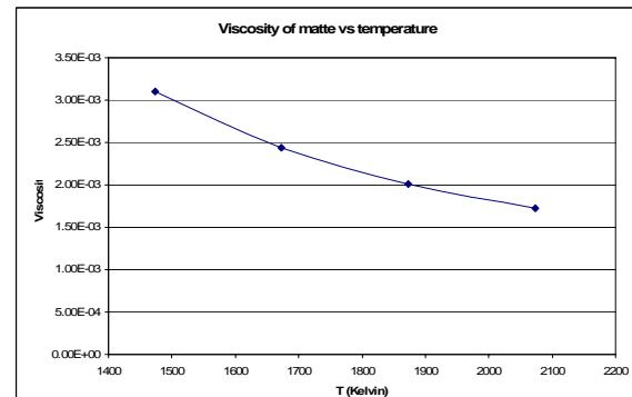
**Figure 14:** Viscosity vs temperature for matte. (Hadley et al. 2006)
