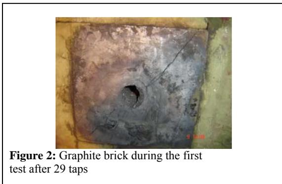
**Figure 2:** Graphite brick during the first test after 29 taps
