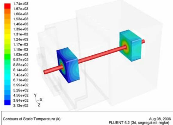
**Figure 8:** The cooling of the matte as it flows through the channel can be seen in Figure 8. It is however seen that the cooling effect on the matte is very little and the average drop in temperature is only 2°C. Figure 8 show the temperature profile of the matte at the outlet with the temperature being at 1739K at the surface but still at 1743K at the centre. The matte inlet temperature was specified 1743K.
