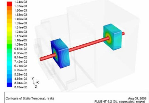
**Figure 7:** The first (left) and seventh tapping bricks thermal profiles showing the seventh tapping module at a much higher overall temperature.
