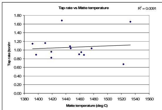
**Figure 13:** Tap rate vs matte temperature determined from plant data. Bath levels are constant between 180cm and 182 cm. No significant correlation exists.
