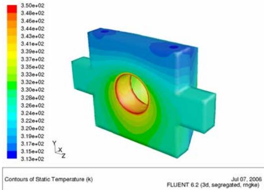
**Figure 6:** Thermal profile through the copper insert. Maximum temperature 77°C.
