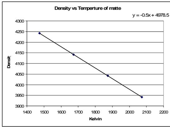
**Figure 15:** Density vs temperature for matte (Hadley *et al.* 2006)
