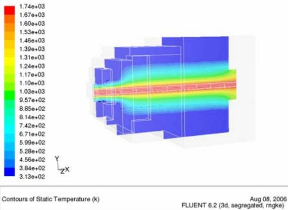
**Figure 4:** A cross section of the tap block showing the thermal profile in the block while tapping
