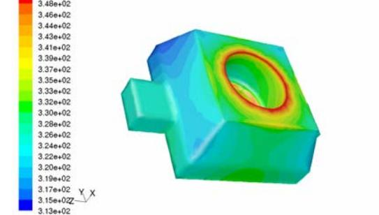
**Figure 6:** Thermal profile through the copper insert. Maximum temperature 77°C.
