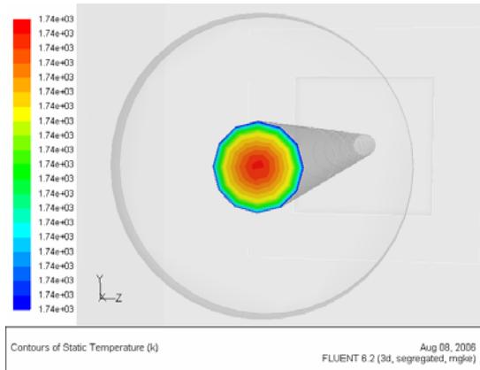
**Figure 8:** Temperature profiles of matte in the tap channel at the outlet.
