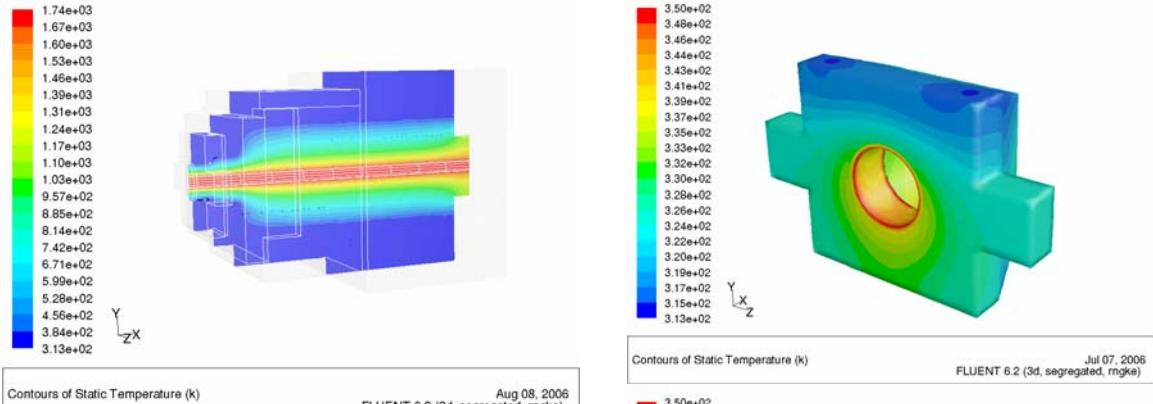
**Figure 4:** A cross section of the tap block showing the thermal profile in the block while tapping
