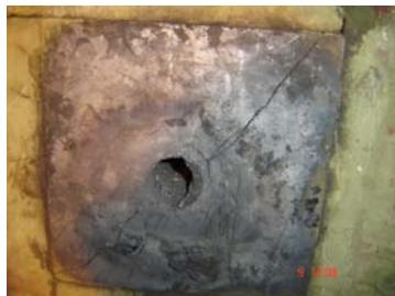
**Figure 2:** Graphite brick during the first test after 29 taps
