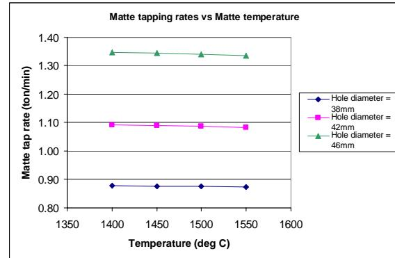
**Figure 9:** Matte tapping rate vs Matte temperature.
