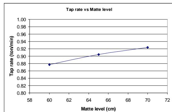
**Figure 11:** Matte tapping rate vs matte levels. Slag level -110cm, Matte temperature - 1450°C, Slag temperature - 1650°C.
