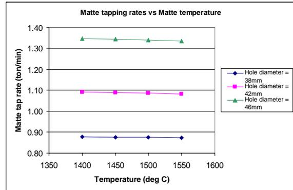
**Figure 9:** Matte tapping rate vs Matte temperature. Matte level – 60cm, Slag level - 110cm, slag temperature - 1650°C
