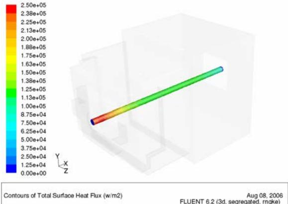
**Figure 5:** Heat flux distribution from the matte. Largest heat fluxes occurring around the front of the tap channel where the copper is closer to the matte.
