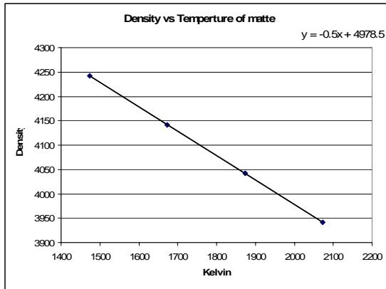
**Figure 15:** Density vs temperature for matte
