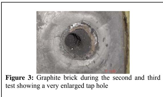
**Figure 3:** Graphite brick during the second and third test showing a very enlarged tap hole
