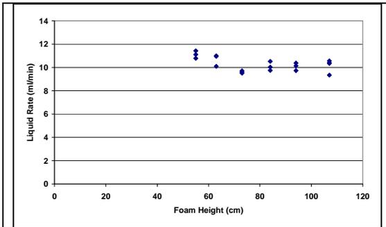
**Figure 3:** The effect of foam height on overflowing liquid rate for a non-coalescing foam, showing that the change in height does not affect the liquid rate.
