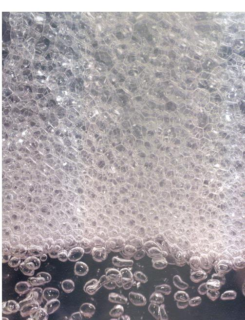
**Figure 1:** Vertical cross-section through a typical flowing foam showing rapid decrease in liquid content and bubble growth
