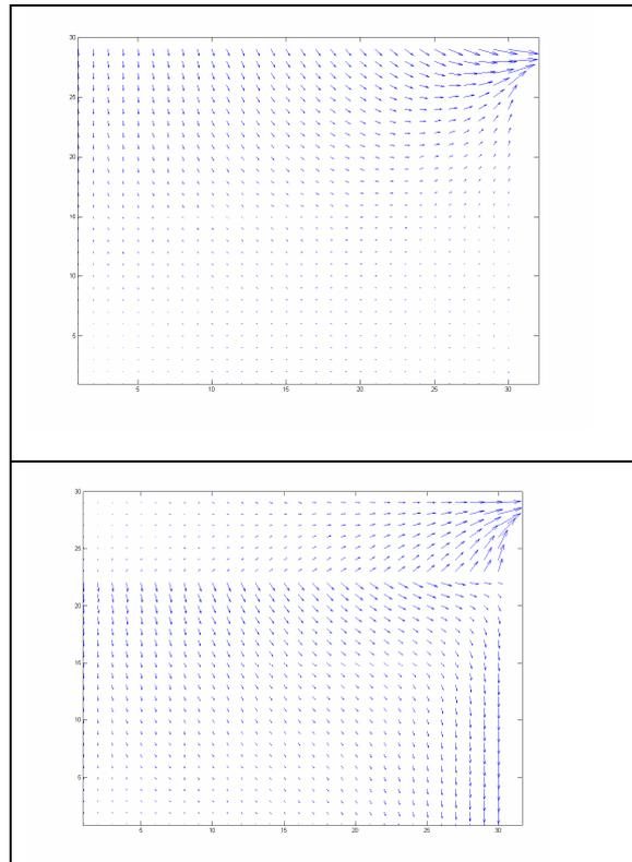
**Figure 4:** Liquid flow velocity vectors for evenly distributed froth washing from the froth surface (top) or inside the froth (bottom).
