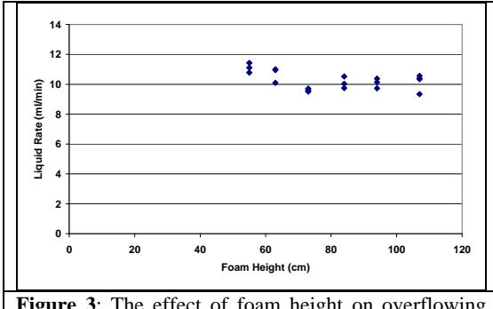
**Figure 3:** The effect of foam height on overflowing liquid rate for a non-coalescing foam, showing that the change in height does not affect the liquid rate.
