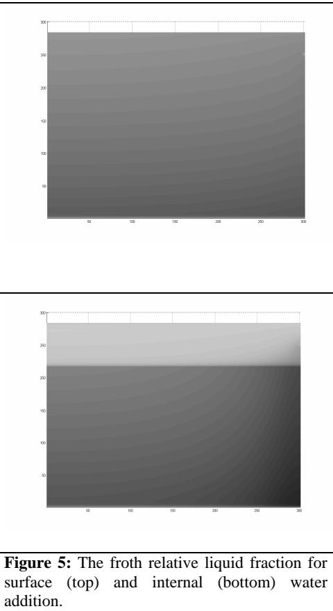
**Figure 5:** The froth relative liquid fraction for surface (top) and internal (bottom) water addition.
