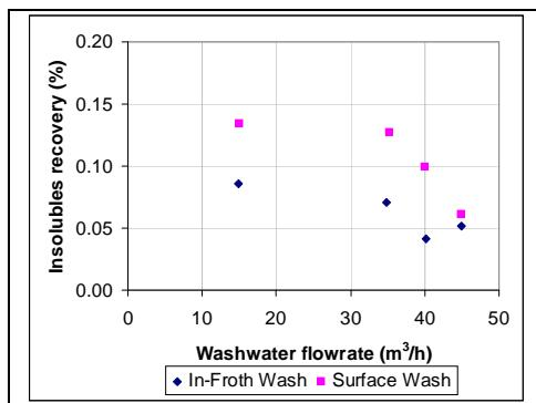
**Figure 7:** Insolubles recovery for surface and in-froth washing showing that at equivalent water rates in-froth washing is superior.
