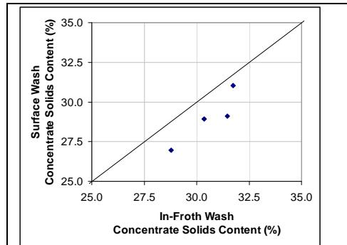
**Figure 6:** Comparison of solids fraction in concentrate for surface and internal froth washing, showing that internally washed froths are drier under equivalent conditions
