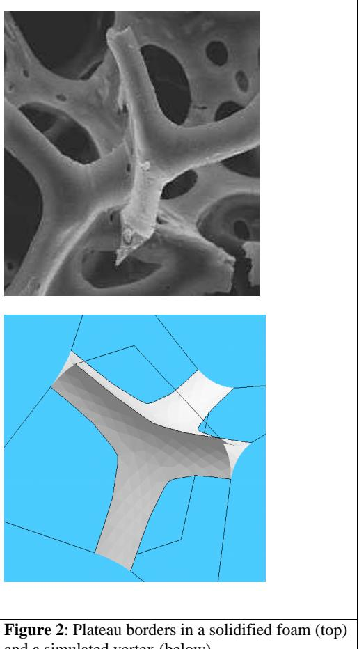
**Figure 2:** Plateau borders in a solidified foam (top) and a simulated vertex (below)
