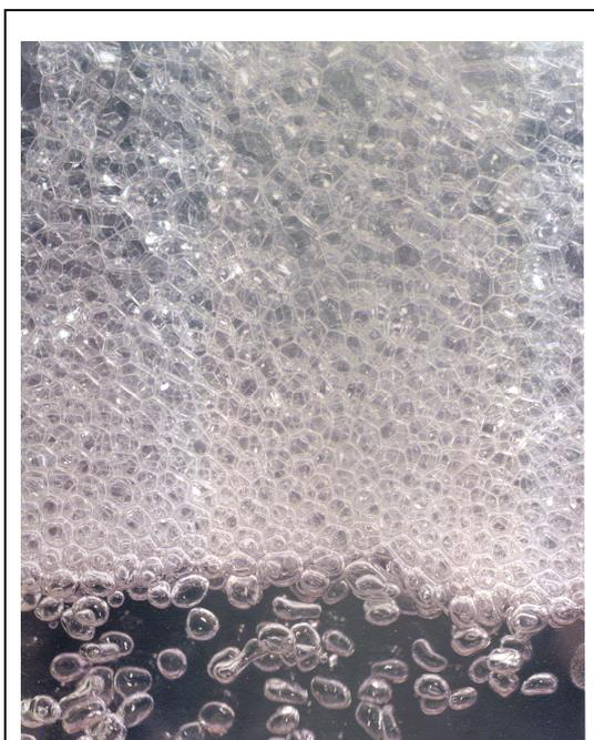
**Figure 1:** Vertical cross-section through a typical flowing foam showing rapid decrease in liquid content and bubble growth
