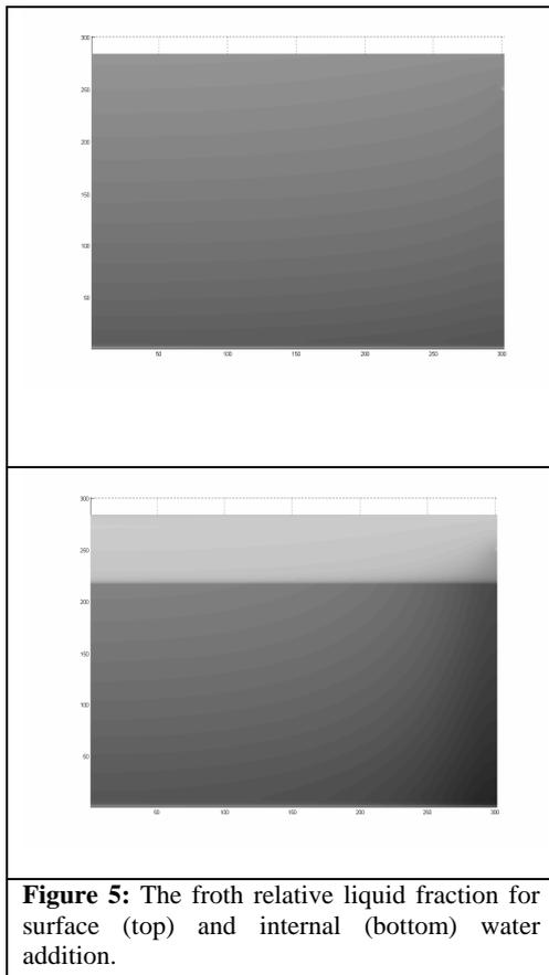
**Figure 5:** The froth relative liquid fraction for surface (top) and internal (bottom) water addition.
