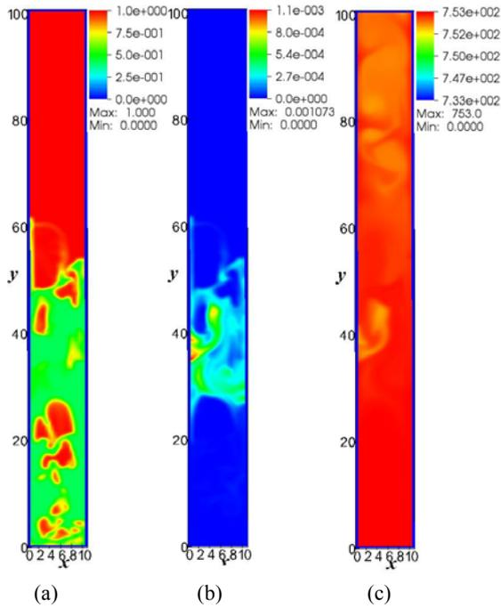
**Figure4:** The contours of gas volume fraction, primary reaction rate and gas temperature; (a) gas volume fraction ( $\epsilon_g$ ); (b) reaction rate ( $R_{g1}$ ); (c) gas temperature.
