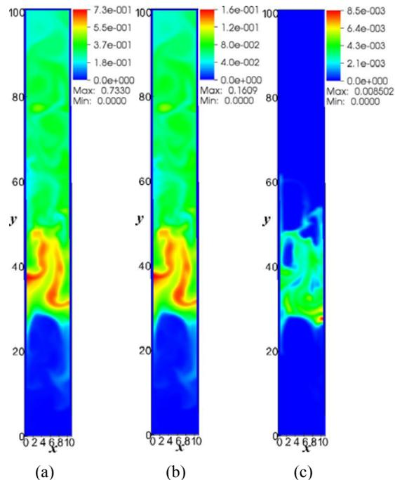
**Figure5:** The contours of products from the primary reaction; (a) mass fraction of condensable gas; (b) mass fraction of non-condensable gas; (c) density of char.
