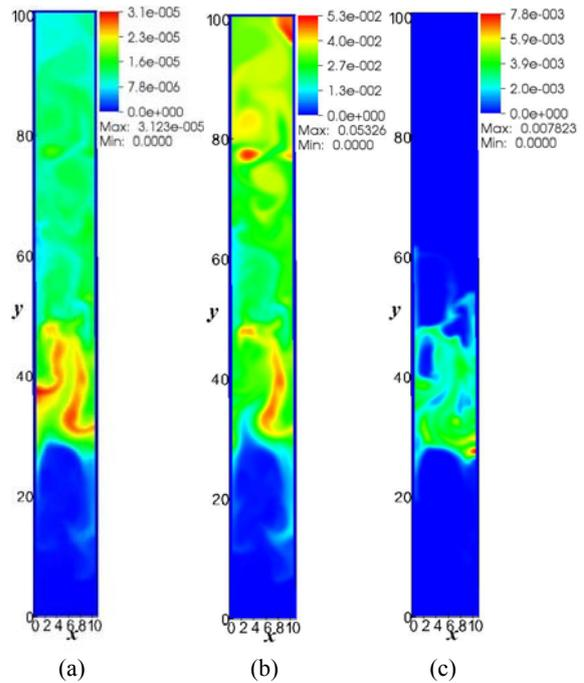
**Figure6:** The contours of secondary reaction rate and products from the secondary reaction; (a) reaction rate ( $R_{g4}$ ); (b) mass fraction of non-condensable gas; (c) density of char.
