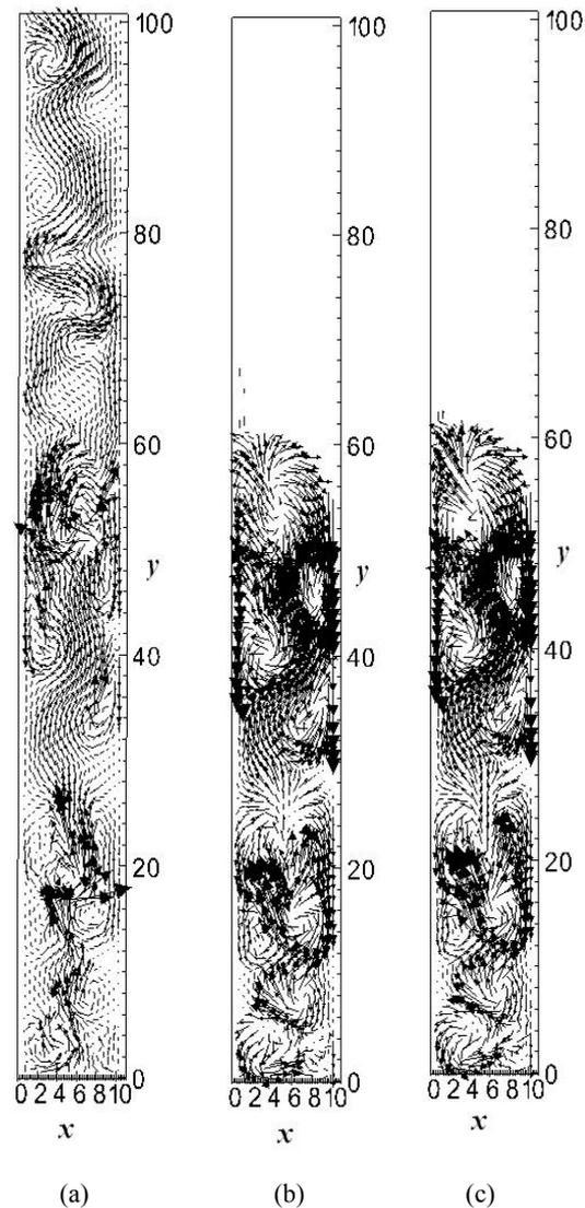
Figure3: The (x, y) velocity vector map; (a) gas phase velocity; (b) solid phase (sand) velocity; (c) solid phase (wood) velocity.
