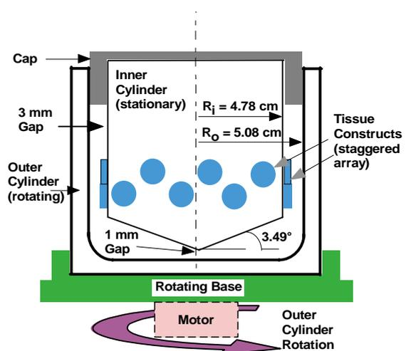
**Figure 1: Concentric Cylinder Bioreactor.** 16 constructs (arrows) are staggered in 2 rows of 8 on the inner cylinder (Saini and Wick 2003).
