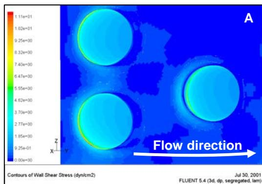
**Figure 7: Bioreactor Steady-State Shear Stress Profiles for 24-Construct Bioreactor** (from (Williams, Saini et al. 2002).
