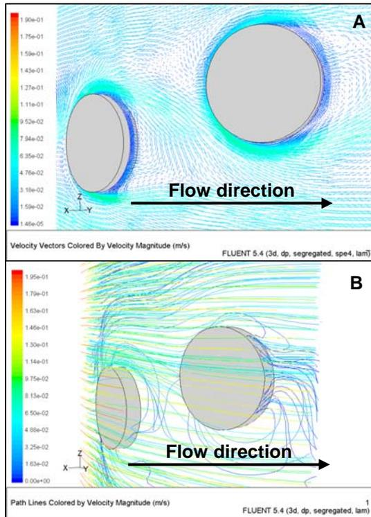
**Figure 4: Steady-State Bioreactor (A) Velocity Vectors (B) and Particle Trajectories** (from Williams, Saini, et. al. 2002).
