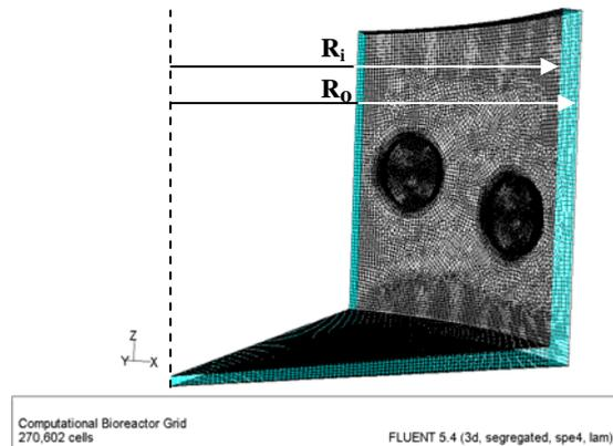
**Figure 3: Bioreactor Computational Grid.** (Williams, Saini et al. 2002)
