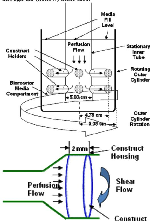
**Figure 9: Perfusion Concentric Cylinder Bioreactor.** Bioreactor schematic (upper panel) and close-up of an individual construct & housing showing construct placement (lower panel).
