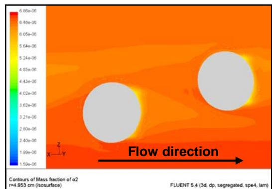
**Figure 6: Bioreactor Oxygen Concentration Profile.** (Williams, Saini et al. 2002).
