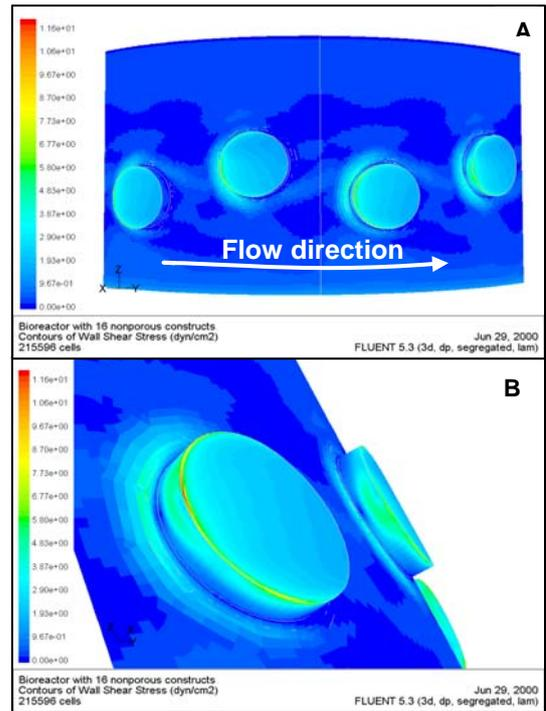
**Figure 5: Bioreactor Steady-State Shear Stress Profiles for 16-Construct Bioreactor.** Panel (B) is enlargement of (A) showing location of maximum shear stress on the leading edge of the upper and lower constructs (from (Williams, Saini et al. 2002)).
