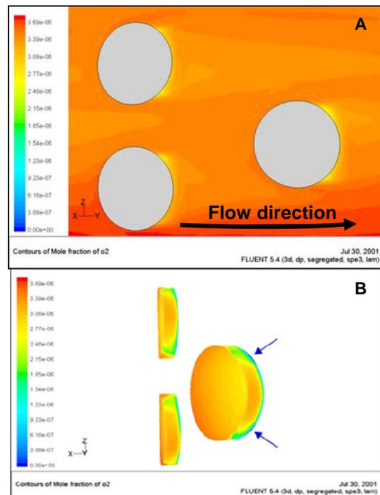
**Figure 8: Bioreactor Oxygen Concentration Profile.** Panel (B) shows small region of oxygen depletion (arrows)(Williams, Saini et al. 2002).
