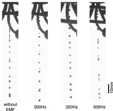
**Figure 6:** Photographs of the formation of the gallium droplets by the intermittent electromagnetic force.
