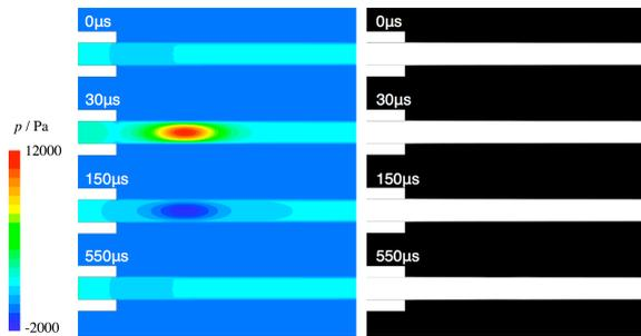
Figure 14: Pressure distribution (left) and the free surface of the jet (right) near the coil (14.7mF).
