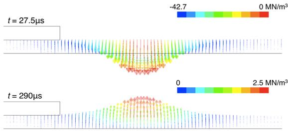
Figure 10: Electromagnetic force field (14.7mF).
