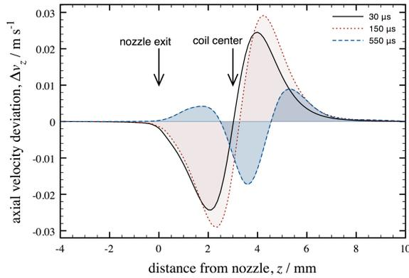
**Figure 15:** Axial velocity deviation from the initial velocity along the center axis.
