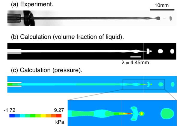
**Figure 8:** Breakup of the capillary jet by a growth of natural disturbance (without an electromagnetic force).
