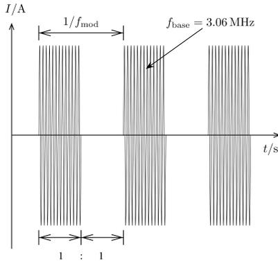
**Figure 5:** Schematic diagram of the modulated current.
