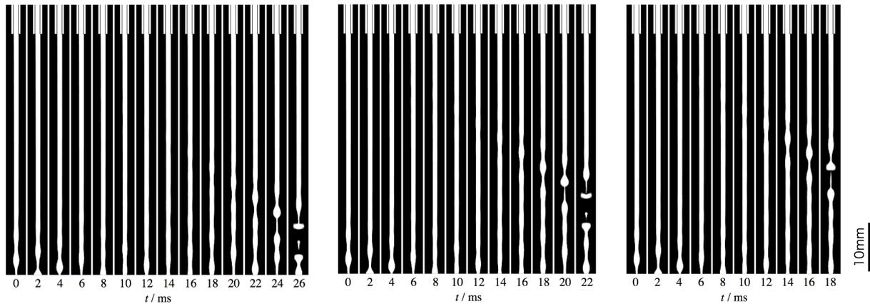
Figure 12: Numerical simulation of the breakup of the gallium jet (left: 4.7mF, center: 10.0mF, right: 14.7mF).
