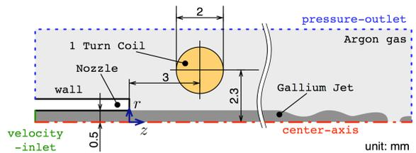
**Figure 7:** Schematic diagram of the calculation domain.
