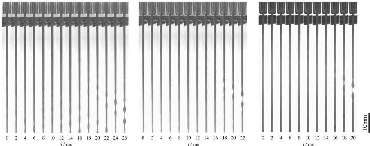
**Figure 3:** Serial photographs of the breakup of the gallium jet (left: 4.7mF, center: 10.0mF, right: 14.7mF).
