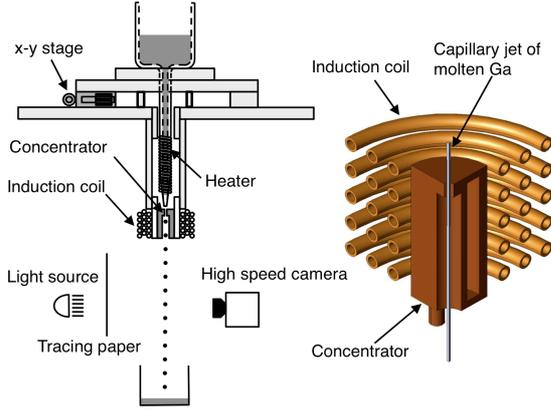
**Figure 4:** Schematic diagram of the droplet generator.
