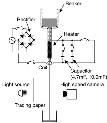
**Figure 1:** Experimental apparatus for the single pulse electromagnetic force experiment.
