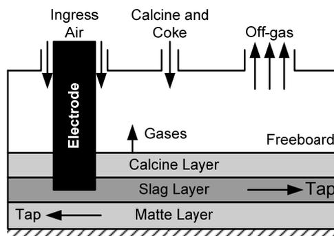
Figure 1: Schematic of the electric furnace.
