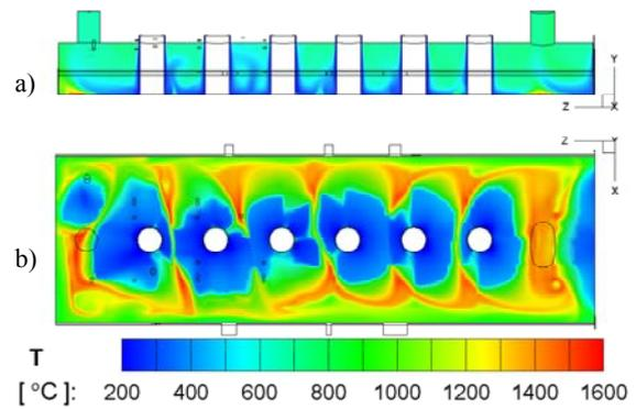
**Figure 8:** Temperature in the freeboard: (a) at a vertical cut along the furnace centre, and (b) at a horizontal cut 5 cm above the calcine top surface.
