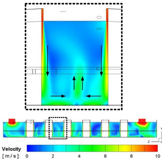
**Figure 7:** Flow velocity in the freeboard at a vertical cut along the furnace centre.
