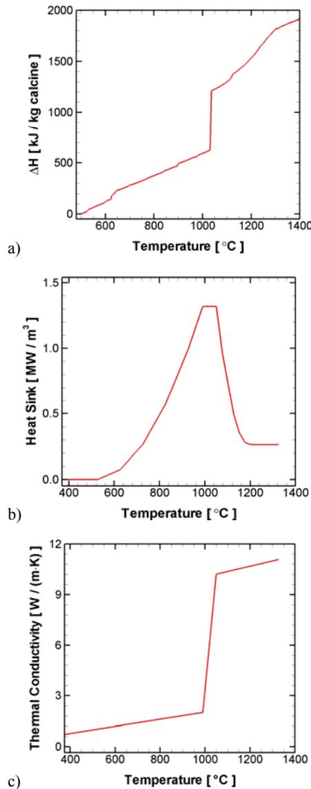
**Figure 4:** For the calcine: (a) enthalpy versus temperature, (b) heat sink versus temperature, and (c) thermal conductivity versus temperature.
