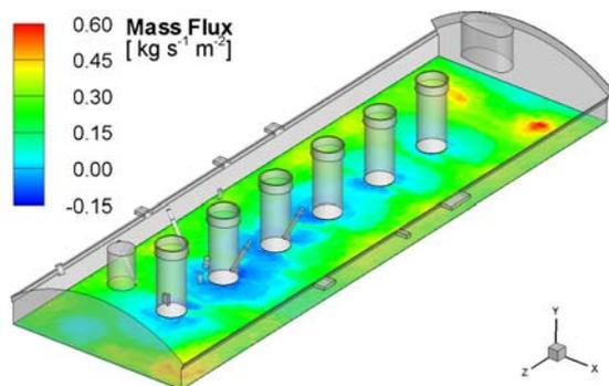
**Figure 11:** Calcine mass flux required to maintain a surface temperature of 550 °C.
