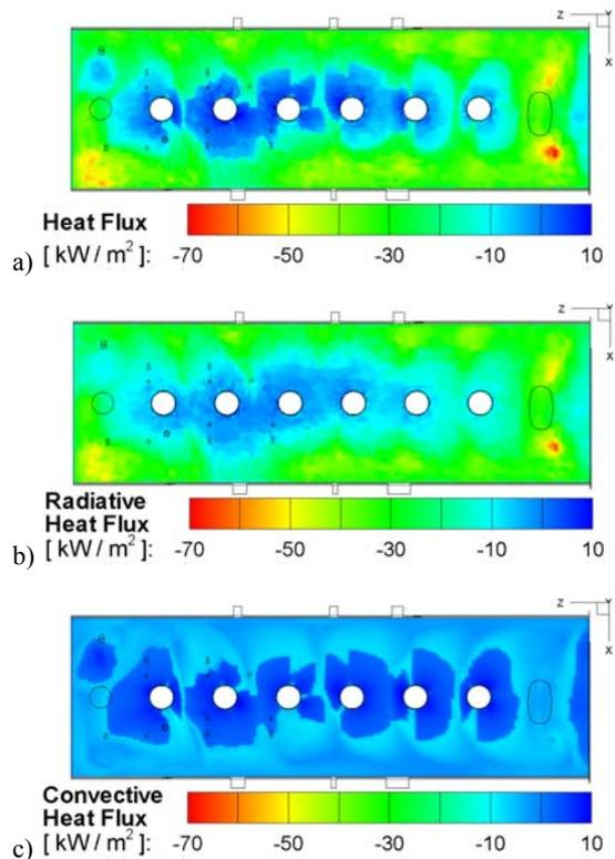
**Figure 9:** Heat flux to the calcine top surface from the freeboard. Negative numbers indicate that the freeboard is heating the calcine and positive numbers indicate the opposite. (a) Total heat flux, (b) radiative contribution, and (c) convective contribution.
