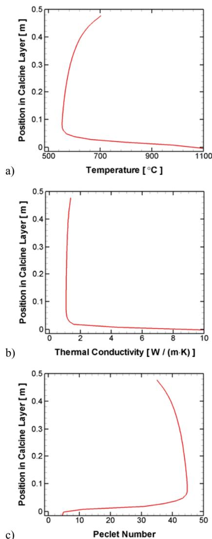
**Figure 10:** Calcine model results: (a) temperature, (b) thermal conductivity, and (c) Peclet number, as a function of height above the slag.
