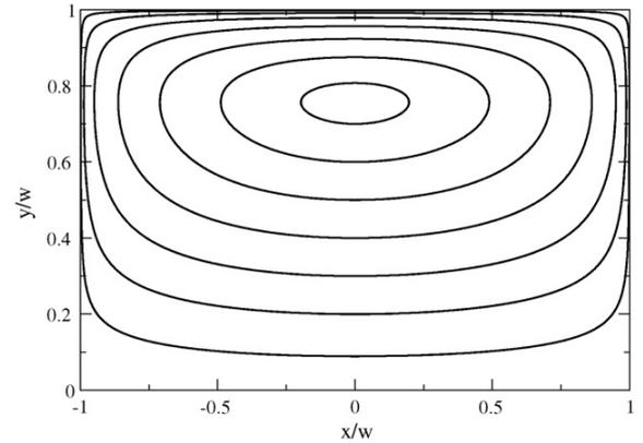
**Figure 3:** Schematic of streamlines at  $O(\alpha)$  velocity flow for the Ostwalde de Waale model (for  $n=0.5$ ). The flow circulates in a clockwise manner around the zero flow point at  $x=0$  and  $y/w=0.76$ , which is the solution of  $f'(y) = 0$ . In the adjacent regions  $-3 < x/w < -1$  and  $1 < x/w < 3$  the streamline pattern is the same except the flow is anti-clockwise about the zero flow point. This streamline pattern is replicated along the entire channel length.
