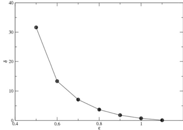
**Figure 4:** Slip length,  $\delta$  as a function of interaction energy parameter between wall atoms and monomers from the molecular dynamics simulations. The dots represent values of interaction parameter which were simulated.
