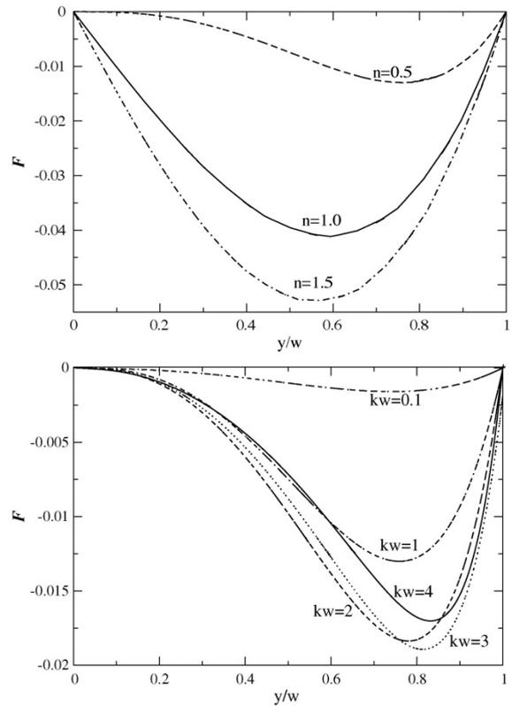
**Figure 1:** Function  $F \equiv kf' / wU^{1/n}$  as a function of  $y/w$  for various  $n$  obtained by solving Eq. (8) (top) and  $n=0.5$  but various values of  $kw$  (bottom).
