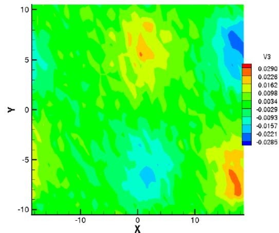
**Figure 6:** Transverse velocity profile for the time dependent body force case for the frequency  $\omega = 2\pi/10$ .
